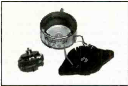
Figure 3. In real motors, the armature is made up of at least three windings, which facilitates the rotation. This is a simplified three-pole motor.
