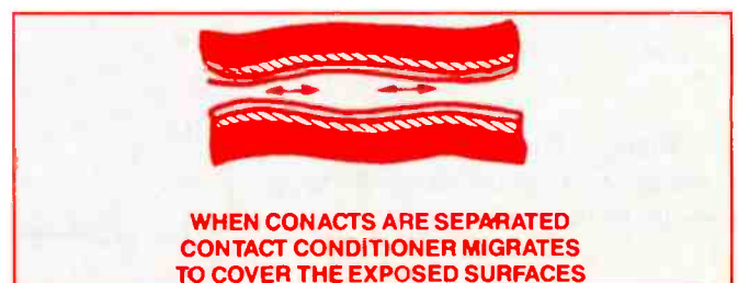
Figure 4. When contacts are separated, the protective chemical migrates to cover the exposed surfaces.
