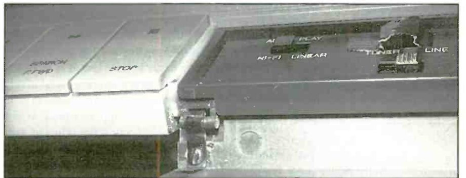
Figure 17. The hinge was repaired using a piece of thin gauge aluminum.
