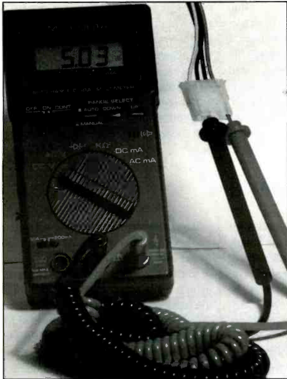
Figure 4. If the computer is dead, turn the power off, remove the cover and locate the power cables coming out of the power supply going to the boards and drives of the computer. Use a DMM to check the voltages.
