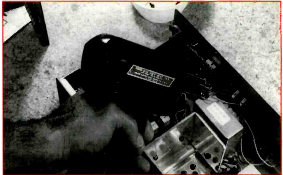
Figure 1. Back in the days of vacuum tubes and hand-wired chassis choice of a soldering tool was easy: a 100-watt soldering gun. It heated up quickly and cooled quickly.
