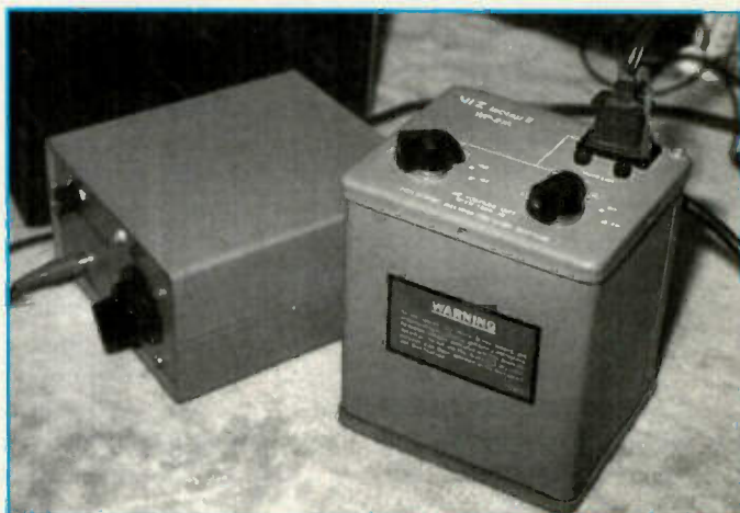
Figure 2. An isolation variable tapped primary and secondary voltage transformer.
