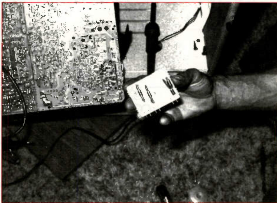
Figure 5. Resoldering all three diode connections upon a SIP diode board solved the intermittent off/on problem in this RCA CTC140-SN chassis.
