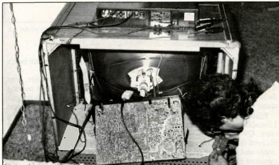
Figure 1. The technician has just removed the diode SIP board to individually check each diode in the low-voltage circuits.
