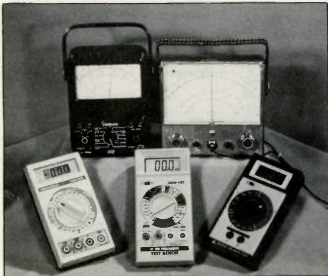
Figure 7. Readings from these five meters are recorded in Table 2, along with the brand and model number of each meter. The black-cased meter is the Simpson VOM, and the square meter with the large meter area is the RCA VTVM. From left to right, the DMMs are the Beckman, the B&K and the American Reliance.
