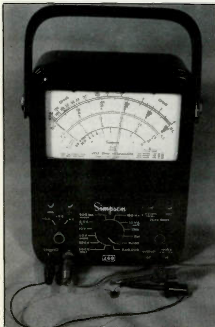
Figure 3. When using the RX100 range of a VOM, connect to base and collector (or base and emitter) with appropriate polarity for the PNP or NPN transistor. A reading of 875Ω is shown by the meter, indicating it is a normal silicon NPN transistor.
