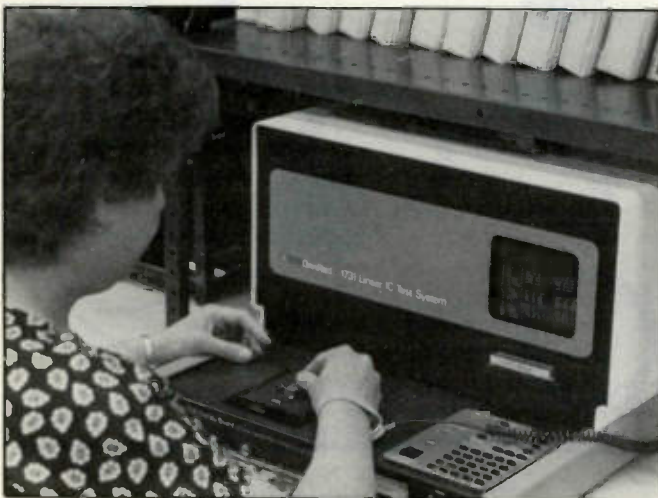
A GenRad linear test set is used to help assure the quality of ECG op amps, comparators, voltage regulators and FETs, just one of many tests designed to ensure the continued success of the electronics servicer.
