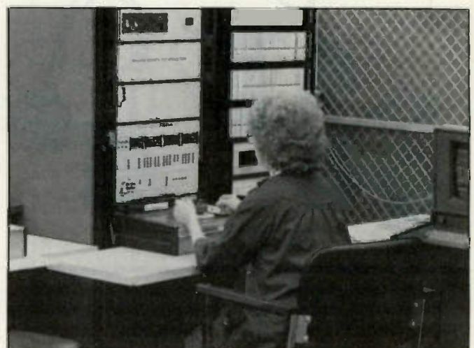
A top-of-the-line, automatic test system is used to verify that ECG discrete components meet quality specifications. As well as testing each device's electrical parameters, the equipment produces hard copy records of many ECG component types.
