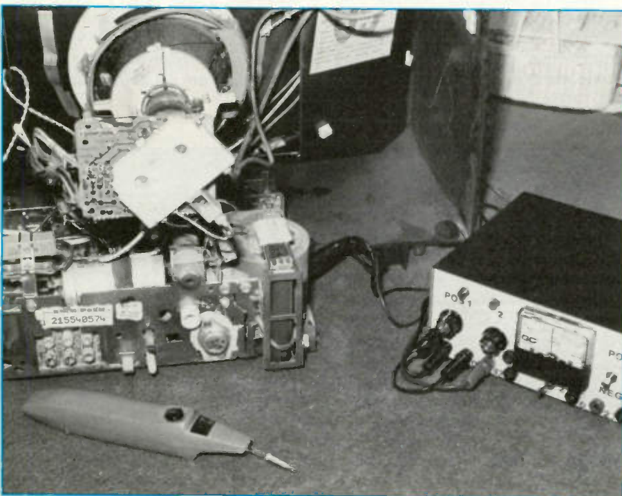
Figure 10. Here a three different voltage sources are found in this power supply with two variable sources and three fixed voltages.
