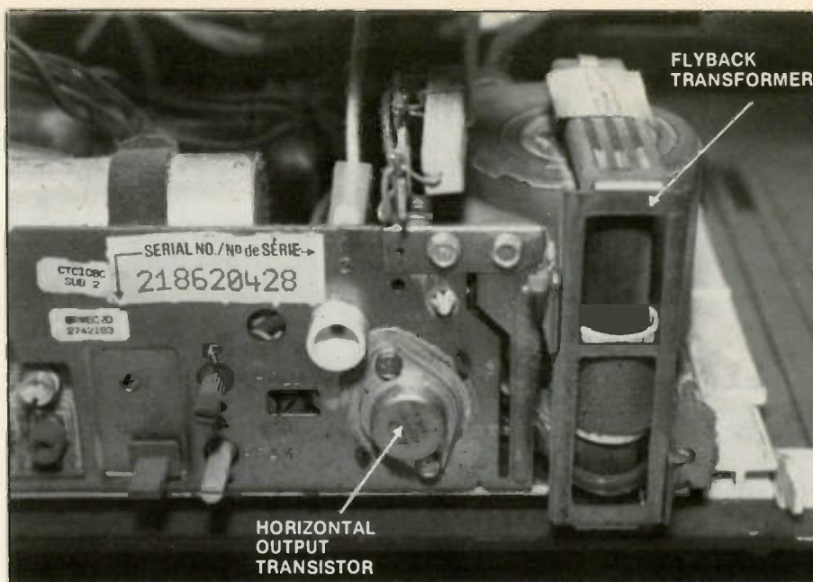
Figure 7. The horizontal output transistor and associated components may cause no start-up or chassis shut-down problems.
