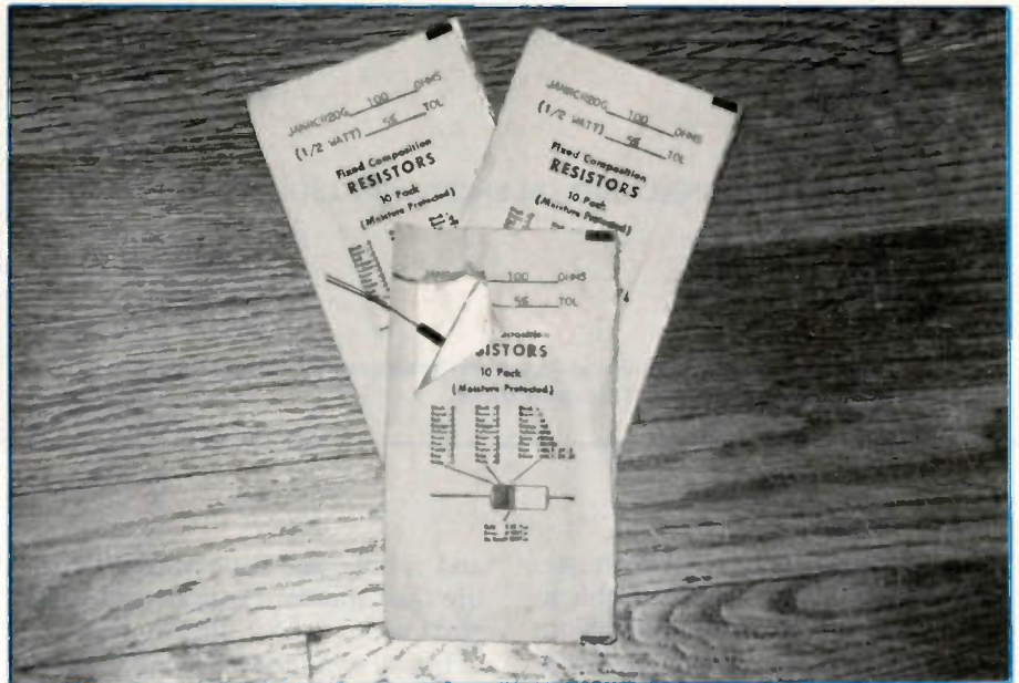
Figure 2. Carbon composition resistors are stored in special moisture resistant packages.
