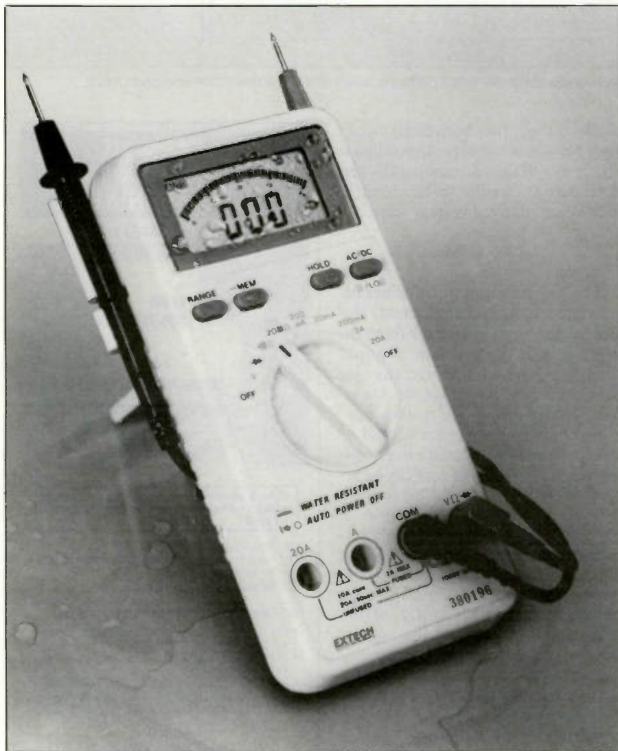
Figure 1. One thing to look for in today's DMM's is their degree of ruggedness. Some meters, such as this one, are designed to withstand harsh environments.
