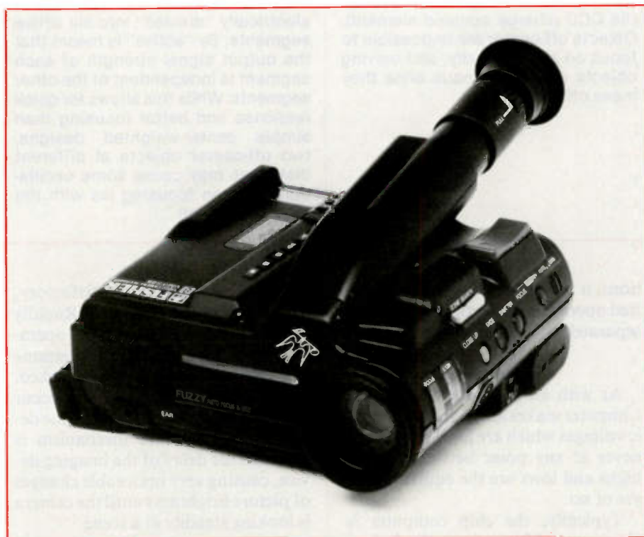
Fuzzy logic provides advanced camcorders such as this with a way to "decide" the most logical object on which to focus. This creates an accurate, human-like focusing system.
