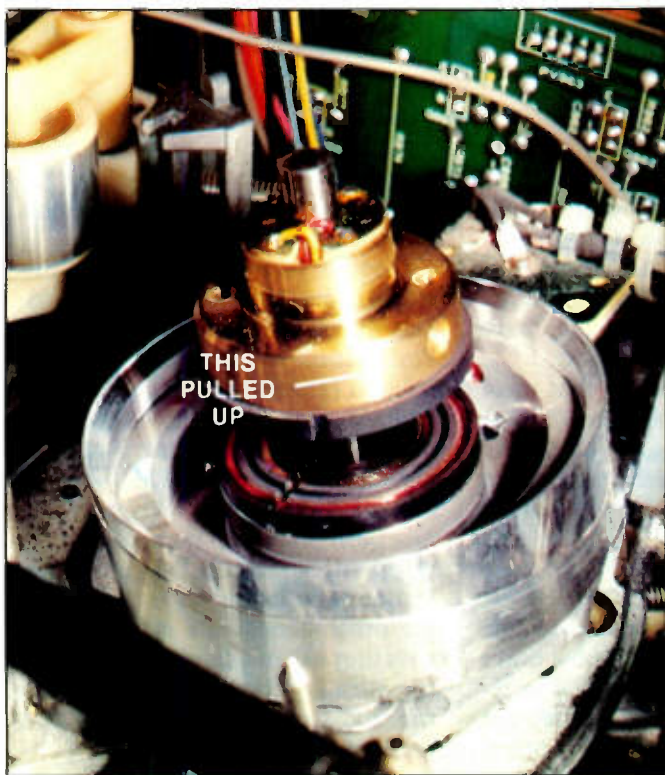
Figure 9. Pull up on the upper part of the rotating transformer to remove it and the cylinder shaft from the VCR.
