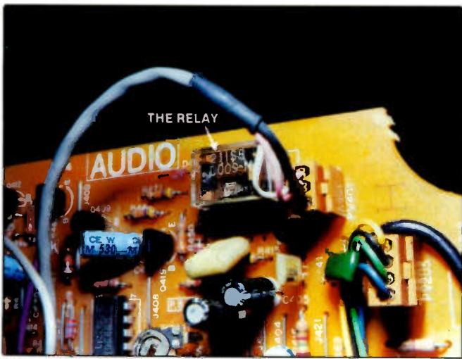
Figure 3. The RE401 relay was sensitive to being tapped by a pencil eraser.
