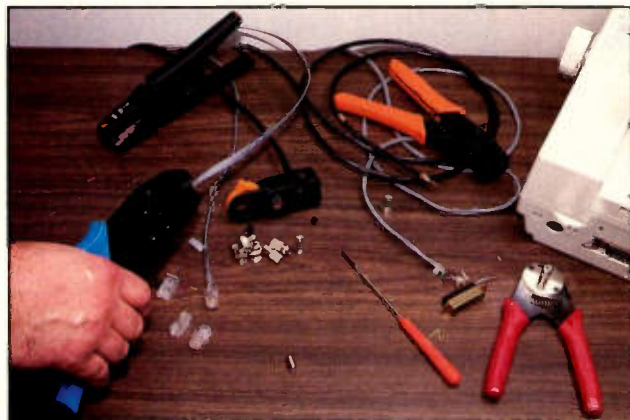
The hazards of non-professional tools are nicked, broken and partially stripped wires that slow down the job.
