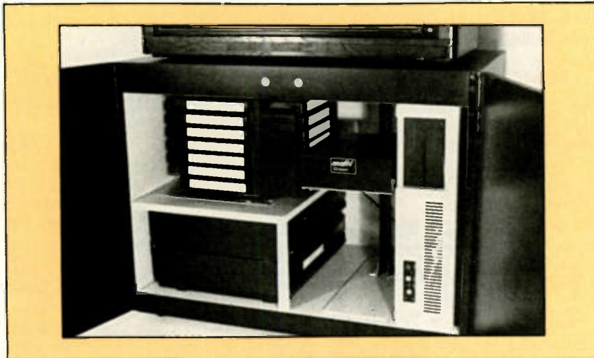
The SmarTV system, stored in a black box the size of a TV stand, contains two VHS VCRs, a personal computer with a modem, and a robot tape changer with a 32-cassette capacity.
