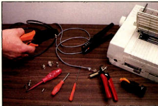
Featuring a full-cycle ratchet, the most efficient tools remain locked until the crimp is precise or the release mechanism is activated.
