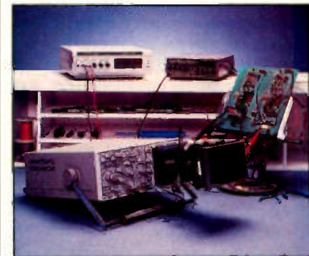
Waveform photography, made easier with a camera bezel on the scope, makes it possible to save waveform information for further study or future reference.
