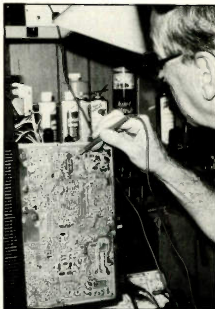
Figure 1. Critical voltage measurements on the audio circuits may locate the defective component.
