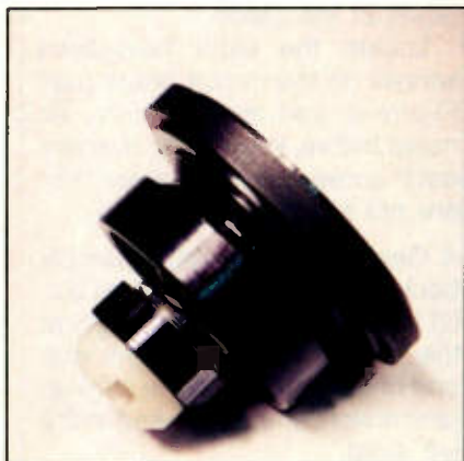
Figure 2. VCR take-up reel. Note the glazed appearance of the clutch tire.
