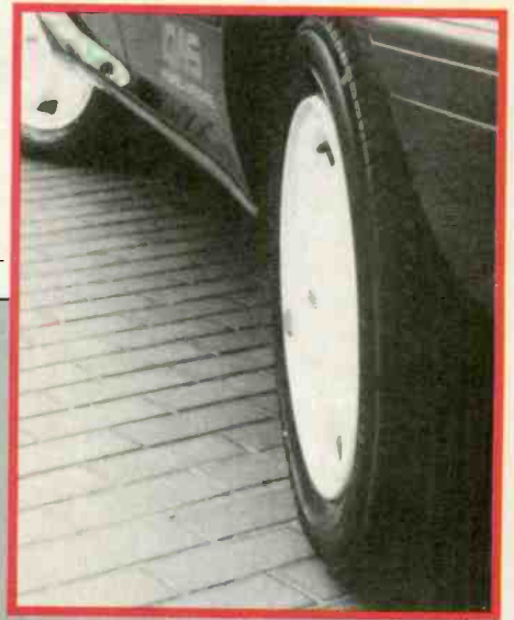
Rear wheels on 4-wheel steering vehicles can turn right or left, responding to both driver's steering and vehicle speed: a maximum of 5° in the opposite direction of the front wheels at speeds under 22 mph, as when parking, significantly increasing vehicle maneuverability. Above 22 mph, rear wheels turn in same direction as front wheels.
