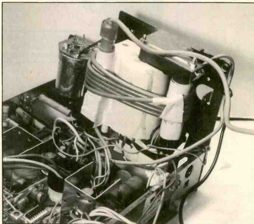
Replacing the defective T400 flyback in Wards GGY-16210C portable restored the high voltage and picture (Photofact 1961-3).
