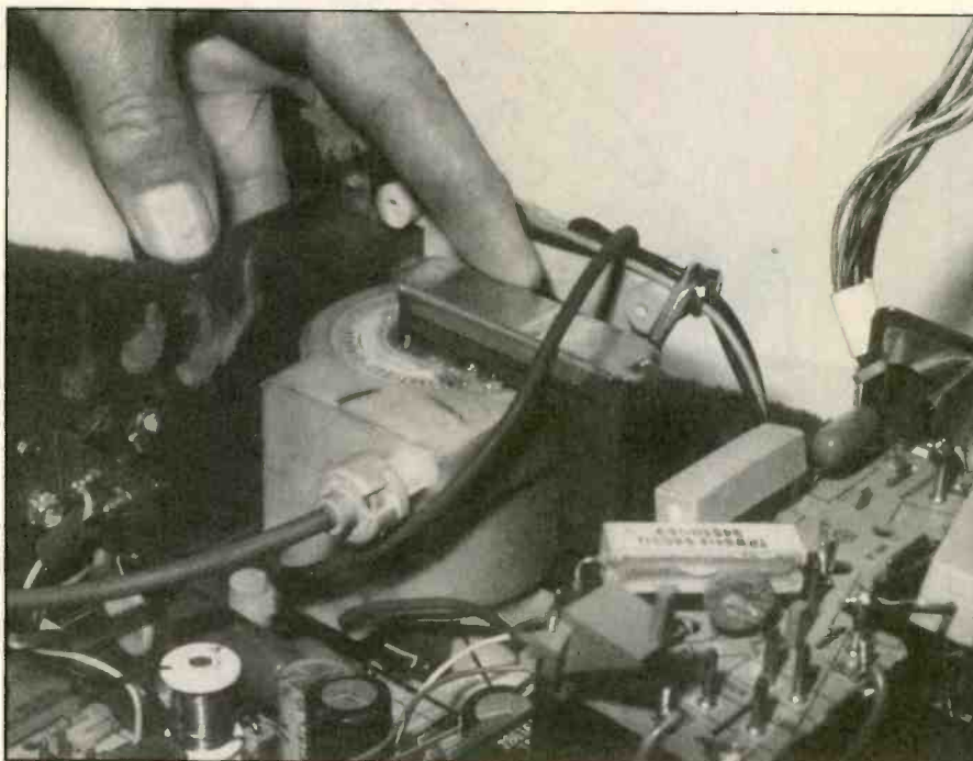
Most flybacks are mounted near a corner (as this one) or at an edge with the horizontal circuitry around them. Most new flybacks are called Integrated High-Voltage Transformer (IHVT) because the HV diodes are inside the flyback.
