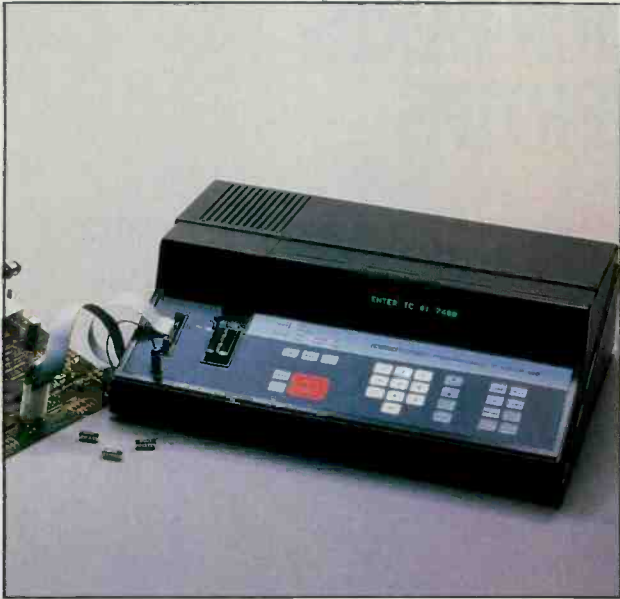
Figure 7. If you plan to troubleshoot a lot of digital logic circuitry, you might want to use an IC tester.
