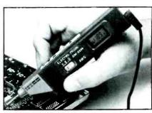
At 63/8"x111/8"x3/4", the DM-6590 is a miniaturized instrument that fits comfortably in the hand and contains a built-in probe tip for one-hand operation. It is designed for reading ac voltage, dc voltage and resistance in tight, hard-toreach areas such as crowded circuit boards.
