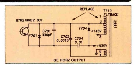
Figure 6. Replacement of the T710 flyback and the C702 retrace-tuning capacitor eliminated the problems of foldover in the center followed by loss of picture. This model uses a regulated power transformer, so it does not require a regulated power supply nor a start-up supply. Neither does it have a recognizable shutdown circuit.
