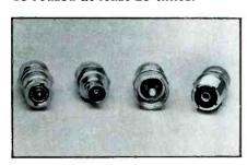
These connectors accommodate popular cable sizes such as RG58, RG59 and RG62 up to RG6U. Solid, foam and air dielectric cables can be used. The center contact has a spring member that accepts the variation in conductor sizes. Maximum jacket size acceptable is about 0.275, depending on the cable braid thickness because the braid is folded back over the jacket before insertion of the cable into the connector.
