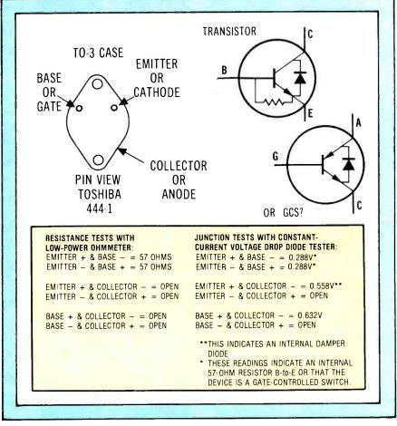
**Figure 3.** According to these resistance and junction voltage-drop measurements, Q601 either is a power transistor with an internal base-to-emitter resistor plus a damper diode, or it is a GCS with a damper diode.
