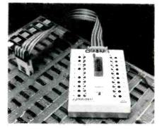
manufacturer. Only a "known good" IC that matches the IC being tested is required.
