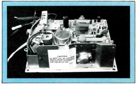
**Figure 4.** This end view of the power/horizontal board shows horizontal-output Q601, the horizontal output transistor, mounted with screws in a socket on the metal heat sink. The Q601 heat sink is connected to hot ground, while the other metal panel (at the left) is connected to cold ground.
