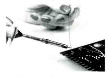
repair. It weighs three-fourths ounce, and is being introduced by M.M. Newman, Marblehead, MA. The tip tapers to 0.10-inch diameter and slides on directly over the heating element.
