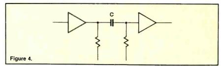
In this application, the capacitor should have a low dissipation factor.
