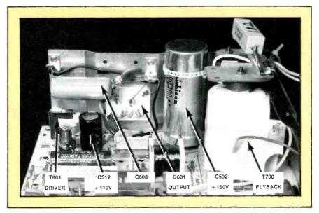
**Figure 5.** Several power-supply and horizontal-deflection components are located by arrows. Notice the plastic band around C502 and a section of the heat sink. This provides increased strength and rigidity to the assembly.
