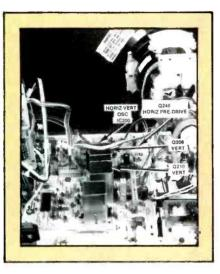
Figure 1. Arrows point out several solidstate components on the signal board. The IC200 horizontal/vertical-oscillator IC is out of sight behind the Q208 heat sink. Q248 horizontal pre-driver transistor is in the corner. Q208 vertical output is on the signal board below its heat sink that is pointed out by an arrow. Also, the Q210 vertical output is on the board below its heat sink. The third heat sink is for Q285, which regulates the + 12.5V supply.
