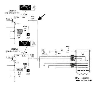
With the TV power unplugged, I located resistor R702 (connected between Q206 collector and the CRT cathode pin 12) and unsoldered the end opposite the CRT cathode. I pierced the insulation of the focus wire near the CRT board with a straight pin. A test lead with a probe in its insulated handle at one end and an alligator clip on the other end was
