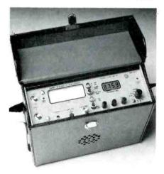
charts, peak detection circuits indicated on a meter calibrated in RMS of peak carrier, input signal level 300V to 1V FSD, digital frequency readout within  $\pm 0.1$ MHz and AM and FM sound detection. Nicad batteries provide seven hours operation per charge.
