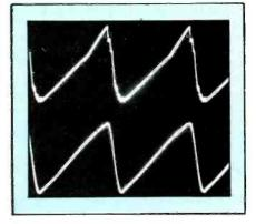
Figure 7. The top trace of the waveform is the combined currents of the output device and the damper diode inside Q601. After it has been affected by the horizontal-linearity circuitry, the horizontal-yoke current has an excellent sawtooth waveshape proving good linearity.
