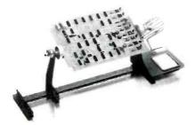
locking end support slides easily to suit board width. Board holders are spring loaded for easy removal and replacement of circuit boards without readjustment. Boards may be rotated 360 degrees, and may be locked at any angle. A specially designed soldering iron holder and tip cleaning sponge are included. The unit is freestanding, or may be mounted to the bench.
