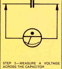
Demonstration of capacitor soakage.
