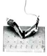
A barrier on the tip prevents shorting between DIPs. The light weight and "fingereze" action permit hook-up to delicate wires where weight and leverage may otherwise damage components. Circle (77) on Reply Card
