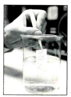
Figure 1. Signal distortion on highperformance electronics is limited by dipping the circuit into Dow Corning 1107 fluid. The component is cured for 15 minutes at 150°C. Improving wetting characteristics of parts reduces the impact of relative humidity on circuitry. In turn, that enhances operating performance of equipment.
