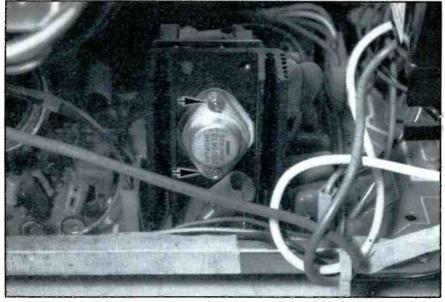
Figure 7. Two nuts (located by arrows) must be removed and the base and emitter leads unsoldered from a small circuit board before TR704 horizontal-output transistor can be removed from the chassis.
