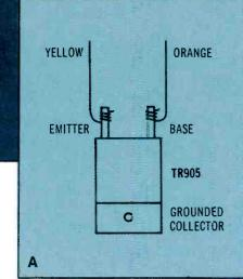
Figure 2A. TR905's base and emitter leads are soldered to colorcoded wires, which must be removed before accurate tests can be made.
