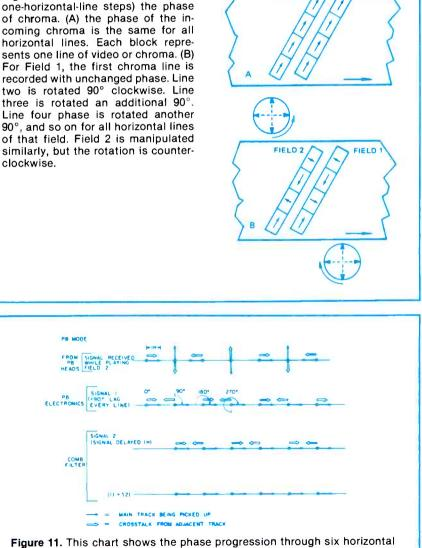
Figure 11. This chart shows the phase progression through six horizontal lines of chroma. After the chroma is sent through a comb filter and the two signals are added vectorially, the crosstalk is canceled, leaving the chroma without interference.
