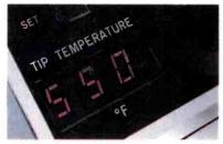
When you need controlled output soldering for sensitive components, you don't need uncontrolled temperature fluctuations at the work station. In the Weller EC Series, the tip temperature is maintained throughout the range of  $350^{\circ}F - 850^{\circ}F$  to within  $10^{\circ}F$ . In addition, an electronic system utilizes thyristor power control with zero voltage thyristor drive. This
