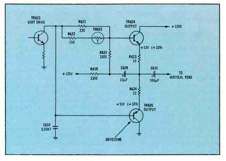
**Figure 10.** Driver and output stages of vertical sweep in the K-Mart model KMC-1920 resemble a complementary-symmetry audio amplifier. Dc voltages in parentheses were measured in one chassis that had an open TR605.
