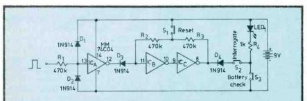
**Figure 1.** Three gates form a latching circuit perfect for troubleshooting alarm circuitry. This circuit latches on positive pulses.
