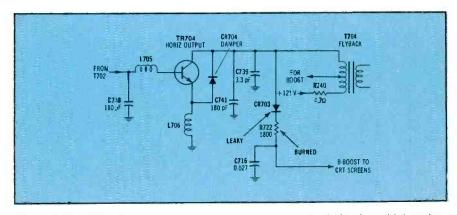
**Figure 6.** The K-Mart horizontal-output stage has no unusual circuits, which makes troubleshooting easier. Boosted-boost components CR703 and R722 have failed in many cases. Of course, TR704 output transistor is the first suspect when sound and raster are missing.
