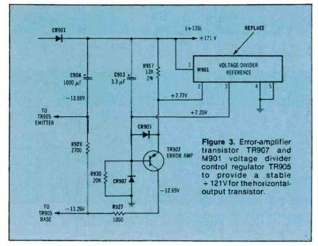
TR905. Replace M901 when the +121V supply measures higher than +125V but no defects can be found. Excessive regulated voltage can produce instant shutdown.
