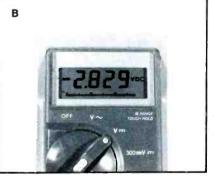
Figure 4. A positive dc voltage (notice the VDC symbol) produces a positive polarity sign on the analog bar graph (A) but no positive symbol before the digital readout. (B) Reversed test probes produce virtually the same digital readout but with negative polarity signs before the digital and analog displays. Automatic upranging occurs slightly above the 3200 count, while downranging occurs at about a 2800 count.
