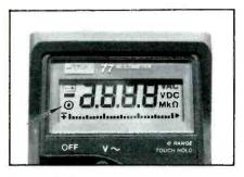
Figure 2. During the internal self-test procedure (which model 77 performs immediately after power is applied to the meter), all LCD symbols, digits, decimals and the complete bar graph are made visible. The arrow points to the manual range-advance symbol on the LCD display. The same symbol is used by model 77 to show when Touch Hold is activated.
