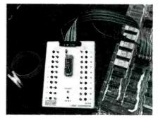
ICs under test are compared to "known good ICs" in circuit and at system speed. Input/output switch settings have been eliminated. Vcc and ground are the only selections required. Model 2074A comes complete and ready to use with reference manual, 20-pin test clip with cable and IDC connector, and 16-pin test clip and cable with IDC connector.
