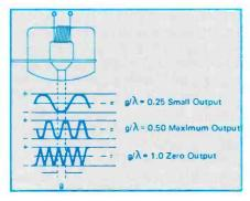
Figure 2. When recording-head current is held constant for all frequencies, the amplitude of the playback-head signal depends on flux strength *across* the head gap. This is in turn dependent on the ratio of head gap to wavelength.
