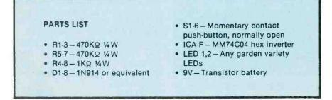
When troubleshooting alarm circuits it is sometimes necessary to detect infrequent logic pulses resulting from false triggering. A simple latching circuit is easily constructed from National Semiconductor's MM74C04 hex inverter IC to observe and "remember" such an event.
