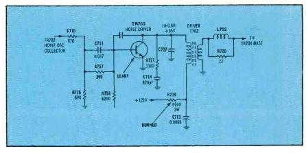
Figure 5. Arrows point to two components that fail most often in the K-Mart horizontal-driver stage.
