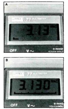
**Figure 1.** Length of the analog bar graph (below the digits) depends on the input signal relative to the range of the digital display. (A) A 3.13Vac signal displayed on the 32Vac range produces a short analog graph of less than 10% of a complete bar graph. A voltage of 16V should produce a 50% bar graph, etc. (B) The same 3.130Vac voltage produces a complete bar graph when the 3.2V range is selected. Notice the Vac symbol that shows the ac-voltage function has been selected.
