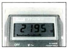
Figure 5. A  $2200\Omega$  resistor tested  $2195\Omega$  on the  $3200\Omega$  resistance range. Notice the corresponding analog bar-graph indication, and the ohms symbol at the right.
