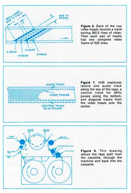
The tape path through a VHS videocassette machine is shown in Figure 8. When a cassette is inserted and the machine adjusted to play or record, the slanted loading pins pull the tape out of the cassette and wrap it around the head cylinder. Posts P2 and P4 guide the tape, keeping it at the correct height and in a horizontal plane.
