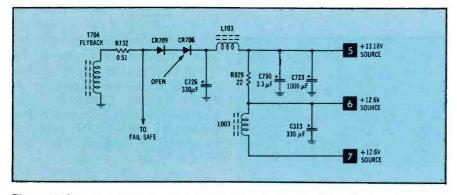
Figure 12. Six low-voltage supplies are produced by rectification of horizontal-sweep power by CR709 and CR706. The 10.72V (CircuiTrace-9) supply is taken through one resistor from the CircuiTrace-5 13.18V supply. R732, CR706 and CR709 have failed in several of these models.
