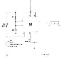
Figure 5c. A 555 Timer IC is another way to provide a stable output pulse even if the input "bounces."
