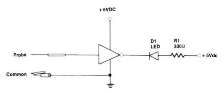
Figure 6. The LED on the *high/low* indicator remains off when a low state is sensed, and turns on when a high state is sensed.
