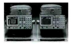
The 338 delivers 32 channels at up to 20MHz. Both models provide glitch capture and three levels of triggering. The models weigh 11 pounds each.
