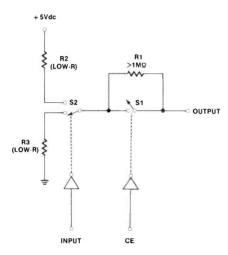
Figure 4a. If no output port is available, one must be provided. In a tri-state output, the third state is a high-impedance in series with the output terminal. particular port.)
