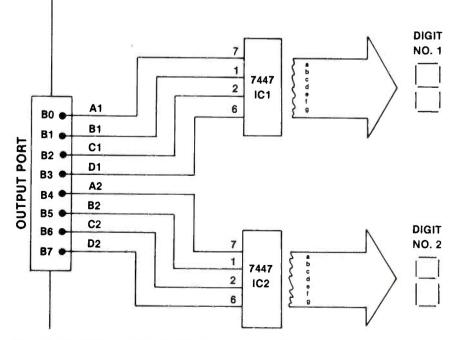
Figure 9. The BCD to 7-segment decoder converts 4-bit binary-coded-decimal number into signals to light the appropriate segments of 7-segment display.
