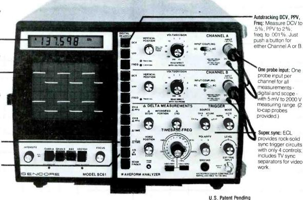
The first scope with push button digital readout. If you use general purpose oscilloscopes for troubleshooting or testing, we can double your present productivity with the SC61 Waveform Analyzer, the first instrument to turn every conventional scope measurement into an automatic digital readout.
