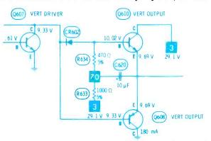
power-output transistor), which showed erratic base-to-emitter conduction. Evidently, the bond inside the transistor case would open from mechanical movement or strain. The problem was an erratic open circuit, but *it was inside a transistor*.
