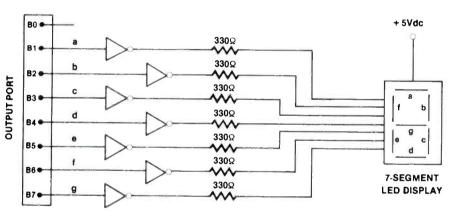
Figure 8. In the case of this latched computer output port, each output line is connected to the appropriate LED segment in the 7-segment display.
