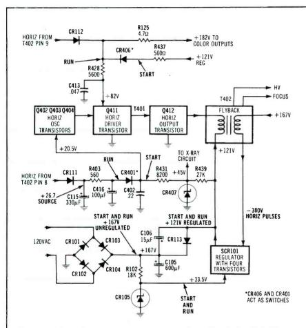
Figure 1. This partial schematic shows several important power supplies.
