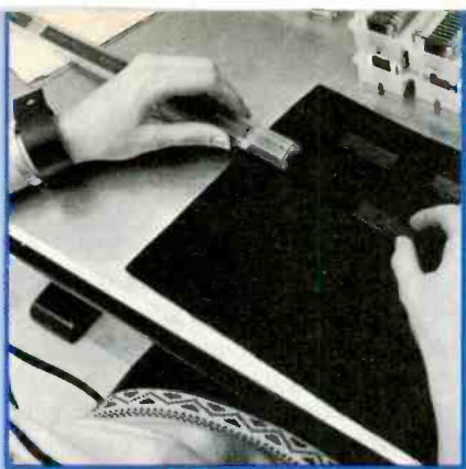
Specially designed carriers of conductive plastic help prevent static electricity damage to DIP components for shipping. Note the conductive foam pad on the workbench. (Photo courtesy of Rockwell International.)
