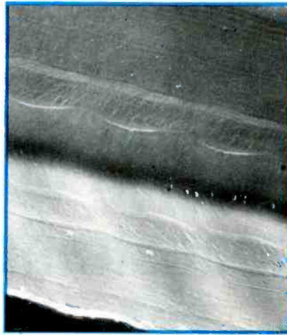
Tracking at 1.5g, an elliptical stylus leaves definite evidence of record wear after 200 hours of use (magnified 3000X).
