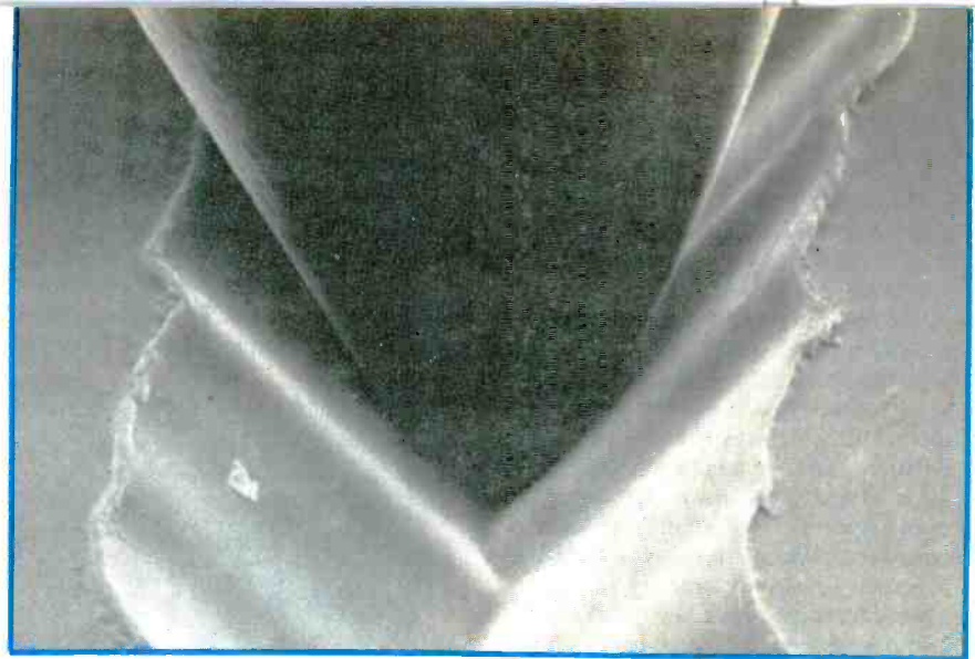
A Stereohedron stylus rests in a disc groove (magnified 2000X).
