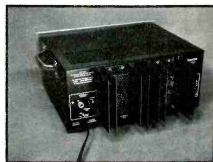
This Dynaco amplifier can be considered typical of the medium-power types manufactured several years ago. No level or tone controls are supplied. Notice the large cooling fins on the rear panel.
