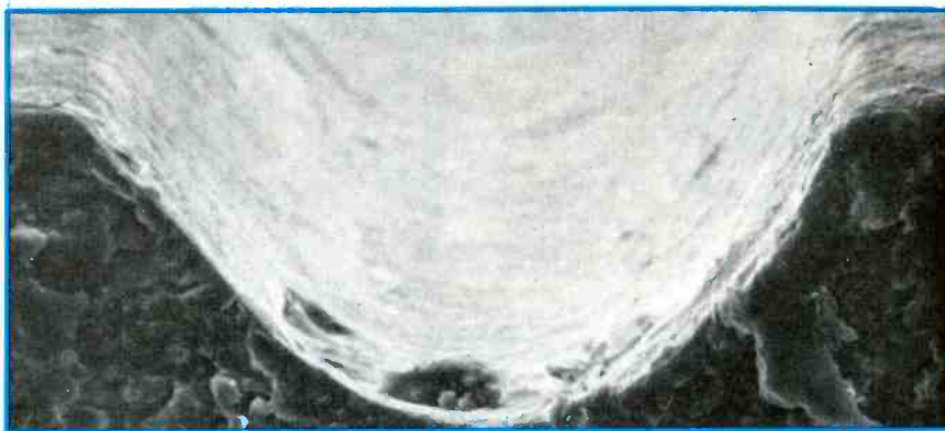
A cross-sectional view of an old 78rpm record (magnified 1000X).
