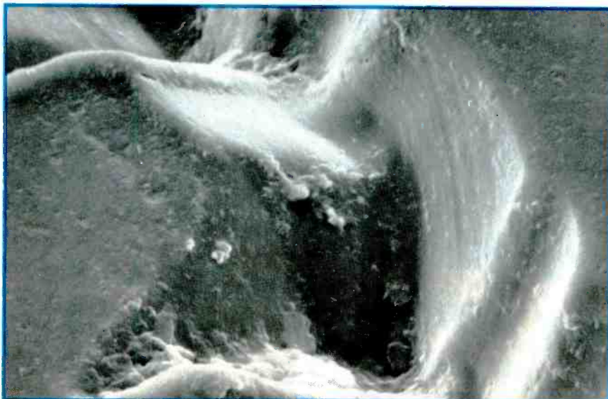
A disc with high groove modulation, as found in many modern recordings. Such modulation would be almost impossible to trace properly (magnified 2000X).
