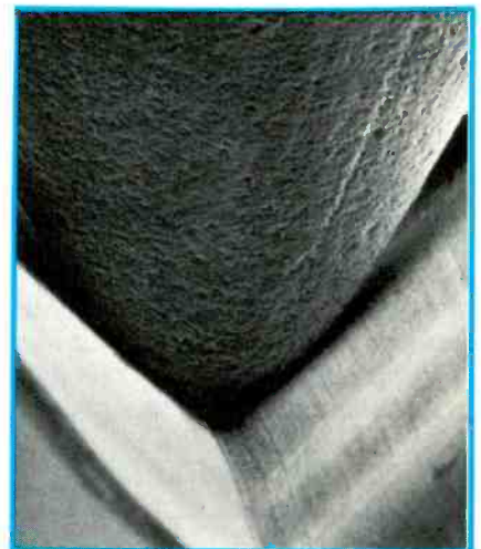
A spherical stylus sits in a phono disc groove. Note the space between the tip and the bottom of the groove. The radius of the stylus is 0.7mil (magnified 2500X).
