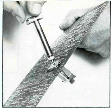
A special bar desoldering iron tip melts the solder holding up to 16 DIP pins. A spring-loaded extractor on the other side of the board removes the component when the solder is properly melted.
