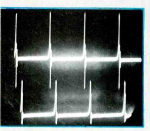
These waveforms illustrate the effects of recording pulses on a type-2, highbias tape at correct type-2 bias and equalization vs. recording with the switch changed to type-1 normal-bias position. The top waveform shows excessive HF response and excellent amplitude when TDK type SA-X new type-2 switch position. This is one proof that a HF boost could be obtained by recording a type-2 high-bias tape as a type-1 normal-bias tape.
