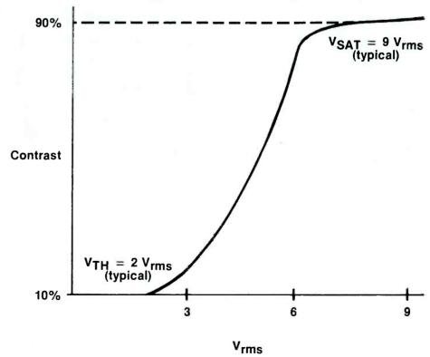
Figure 2. Typical voltage/contrast characteristics of a dyed phase-change oscilloscope display.
