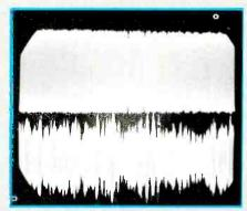
cidence of drop-outs (times of low outbut) when a 8kHz sinewave was recorded and played on a good-quality cassette tape. Compare that waveform with the jagged one below produced by an Avanti brand tape. This was the worst case of drop-outs found during the extensive tests. Excessive drop-puts reduce the HF response and can cause a ragged sound quality. The scope trace was a single sweep that required 0.5s.
