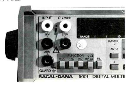
**Five banana jacks** accept a *guard* ground and four jacks for 4-wire resistance measurements (when desired). The two *input* jacks are for all five functions.
