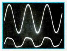
These waveforms prove the futility of using a low-sensitivity tape and trying to compensate by recording at a much higher level. Photo 1 shows the 0dB, 400Hz recording signal (top trace) and the -6.5dB playback signal (bottom trace). The tape had a weak signal when played, so the recording level was increased to +9dB (top trace of Photo 2) and a 0dB playback level was obtained (lower trace). However, amplifier clipping and tape compression added unacceptable distortion.
