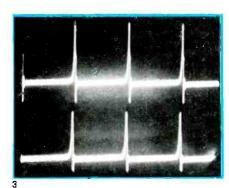
trace shows the good performance of a Fuji metal tape, while the bottom trace shows almost identical results from a Memorex metal tape. In Photo 5, three Radio Shack tapes are compared. The top trace is Supertape Gold, which has good
