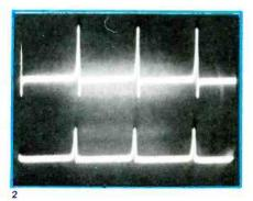
waveform shows the sensitivity winner (Maxell XL1S) having the highest amplitude and good HF response. The lower waveform was made by a high-speed duplication tape of good quality; it shows fairly good amplitude and response. The Photo 4 top
