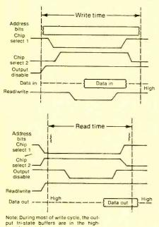
Figure 6. Writing into, or reading out of a RAM requires that several waveforms be present with the proper polarity, amplitude, waveform, and at precisely the correct time.
