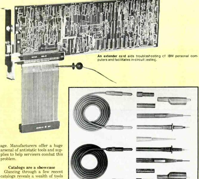
A test lead set enhances versatility of multimeters.
