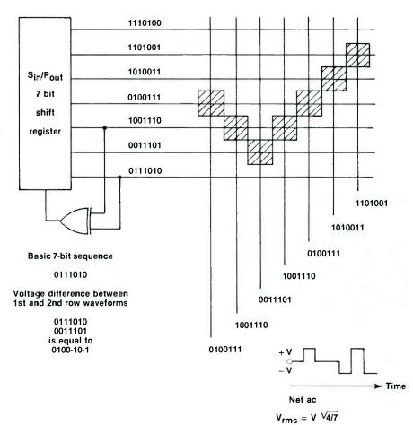
The generation of row waveforms for a 7-row matrix.
