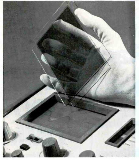
This liquid-crystal, 128-by-256 matrix incorporates the dye-phased change effect to enhance brightness and contrast of a display over a wide variety of ambient light conditions.
