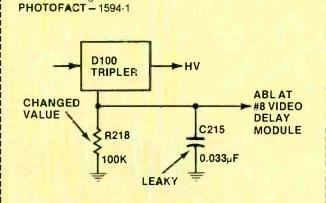
Symptom – Excessive brightness with retrace lines, and no control of brightness
