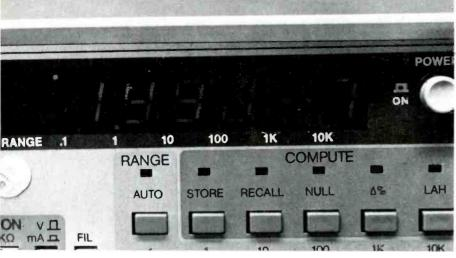
A D battery measured + 1.49097Vdc, and the display was stable. Notice the added LED segment at the bottom of the 4 digit. The same display shows letters, also.
