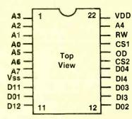
Figure 2. The pinouts for RCA CDP 1822 256-word by 4-bit MOS static RAM are shown. A1 through A7 are seven address inputs for a 7-wire address bus. DI1 and DI4 are four data inputs, from a bidirectional data bus. D01 through D04 are four data outputs, to a bidirectional data bus. CS1 and CS2 are chip-select inputs. RW is the Read/Write input. OD is the Output Disable used to control output to bidirectional data bus. V<sub>DD</sub> is the drain supply voltage. VSS is the source supply
