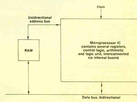
Figure 1. The memory (RAM in this case) is connected into the system by means of multiple-wire buses.
