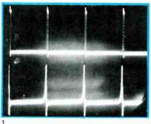
private-label SBC tape. The waveform shows slightly lower amplitude and HF response than for TDK type AD. The lower waveform shows decreased amplitude and poor HF response from a low-priced "white" tape. In Photo 3, the top
