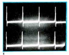
amplitude and fair HF response; the center trace, from Realistic Low Noise, shows moderate amplitude and fairly good HF response; the bottom trace illustrates the weak amplitude and poor HF response of Concertape. These waveforms prove
