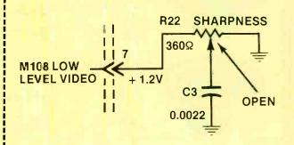
Symptom — Appears as AGC trouble, insufficient brightness or a weak CRT Cure — Check R22 sharpness control and replace it if open
