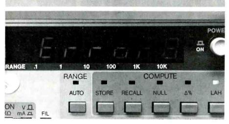
Several operator mistakes and internal-circuit malfunctions will activate a code on the LED display, as shown here where the screen reads *Error 8*.
