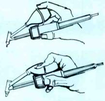
A combined bulb and soldering iron frees one hand to remove the desoldered component.
