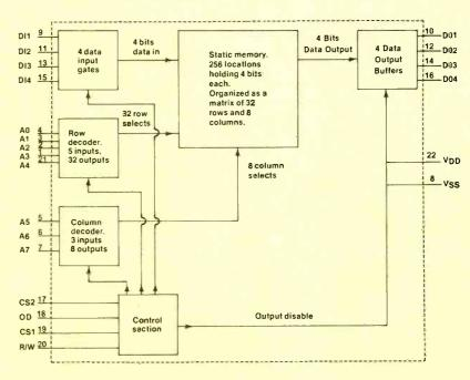
Figure 3. A simplified version of the internal organization of a 256 X 4 static RAM.
