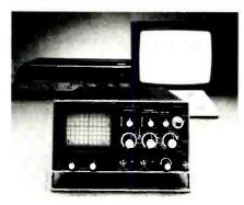
waveform to enable easy and accurate alignment of VCR, VHS, BETA and videodisc recorders. By pushing two buttons, the instrument automatically triggers the TV line, enabling the operator to select each individual line of the TV waveform to be investigated on the CRT display.
