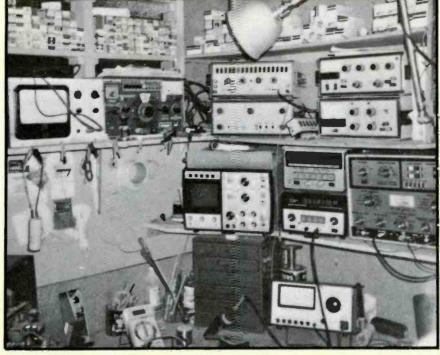
C.A. Honey's main work bench is "L" shaped, with major test equipment at the right, on the short side of the "L." The arrangement allows convenient access to the equipment controls without test leads and cables resting on the televisions and other items under repair.
