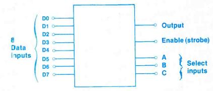
Figure 2A. An IC multiplexer with terminals labeled.
