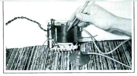
Figure 8 This RCA flyback was replaced after arcing sounds were heard coming from it. After the flyback was removed, a cracked area could be seen in the plastic covering of the high-voltage winding. Evidently the internal arcing had damaged the plastic.
