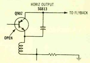
Symptom - B + is normal, but no raster or sound Cure - Check Q902 horizontal-output SCR, and replace it if open
