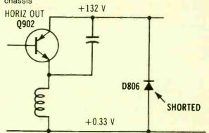
Symptom - + 135V supply shorted to ground, no sound or picture Cure - Check damper diode D806, and replace it if shorted
