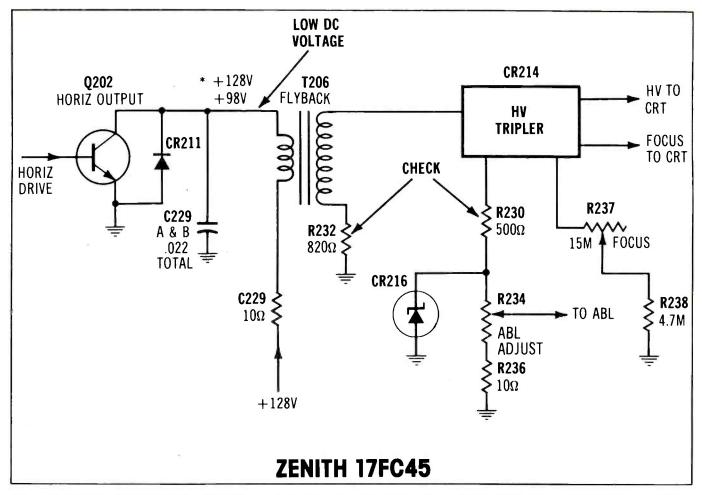
Figure 3 A defective CR214 tripler in a 17FC45-chassis Zenith reduced the high voltage and the Q202 collector voltage. Resistors R232 and R230 should have their resistances tested following any tripler or high-voltage overloads.
