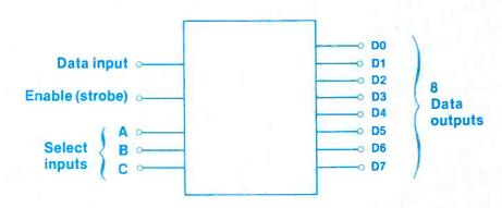
Figure 2B. An IC demultiplexer with terminals labeled.
