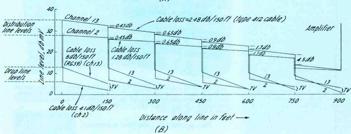
The number of amplifiers that may be cascaded in a cable system depends upon the signal-to-noise ratio of the amplifiers.
