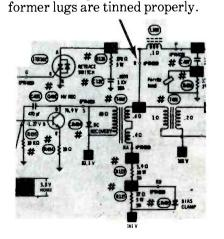
We traced the copper wiring on top of MAH001. Between T401 and T402 is lug R, and an erratic connection was found there. After this lug and the transformer lugs were soldered carefully, the intermittent was cured.
