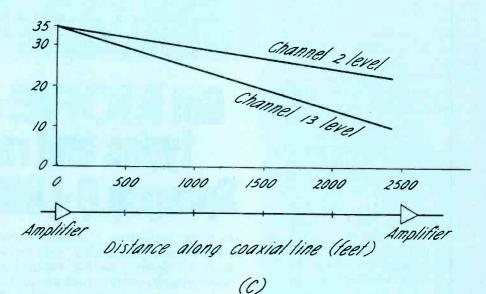
The TV signal suffers losses along the cable proportional to both ambient temperature and the frequency of the signal. (Illustrations courtesy of CREIIMcGraw Hill.)
