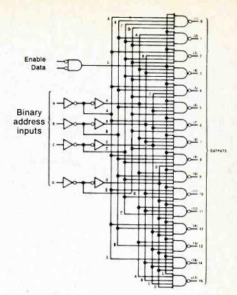
Figure 3A. A 74154 decoder/demultiplexer schematic.
