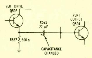
Symptom - Vertical foldover at bottom of picture Cure - Check capacitor C522, and replace it if the capacitance is incorrect or leakage is excessive
