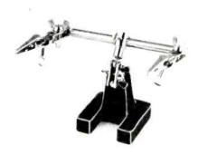
tire assembly is mounted in a heavy cast-metal base to provide stability during use.
