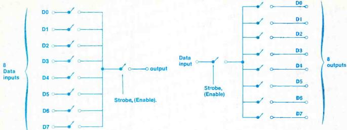
Figure 1A. The elementary switch equivalent of an 8-input data selector/multiplexer.
