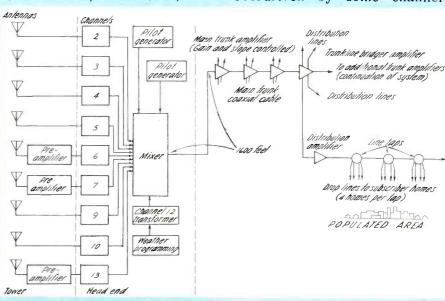
Figure 2. Part of a typical cable TV system.
