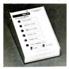
more than 5W. When a disturbance appears on the line, the unit sounds an audible alarm and lights any of six red LED indicators to identify the power problem.
