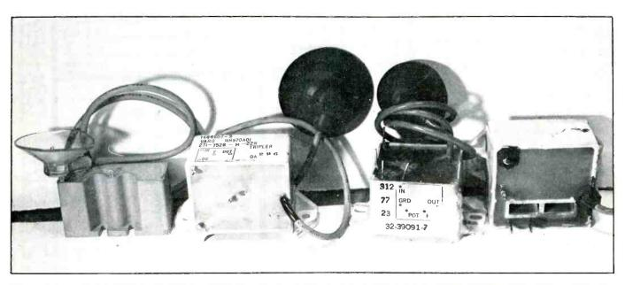
**Figure 1** Four original triplers are pictured. From the left, the first is from an Admiral color receiver, the second is from an RCA, the third was taken from a Sylvania (it shows an attempt to stop an arc) and the fourth is from a Zenith television. Dimensions and mountings vary according to models.
