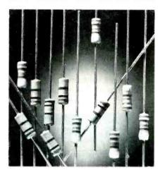
ceramic coating. This construction also provides stable resistance to normal operating current despite variations in ambient temperature, humidity or voltage.
