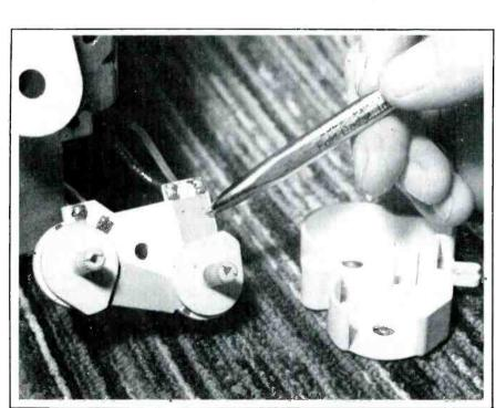
Figure 5 Spots and lines in the picture, caused by receiver arcing, can originate from the anode lead or the focus control. This thick-film, focus-control wiring (from a CTC46 RCA) generated picture interference from arcs.
