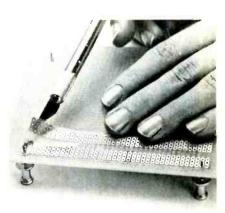
The E-Z Circuit features pressure-sensitive copper component mounting configurations, donut pads, tape and Cut 'N' Peel copper sheets for building, modifying or repairing PC boards.
