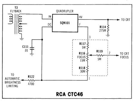
Figure 4 Internal arcing was found in the quadrupler of an RCA CTC46A chassis. Check the Photofact listings to be certain a proper rectifier unit is ordered for replacement. Triplers and quadruplers have the same outward appearance.
