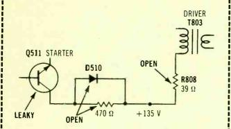
Symptom - No sound, picture or start-up Cure - Check R808, R556 and diode D510, and replace if open. Also, check Q511 for leakage.
