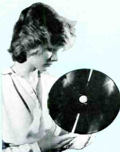
Figure 1. The videodisc is 12 inches in diameter and 70-mils thick. The TV signal is recorded in a spiral groove (10,000 grooves per inch—about 40 times as many as on an audio-LP record). The disk material is made electrically conductive by the addition of 15% of finely divided carbon. In playback, the disk rotates at 450rpm.
