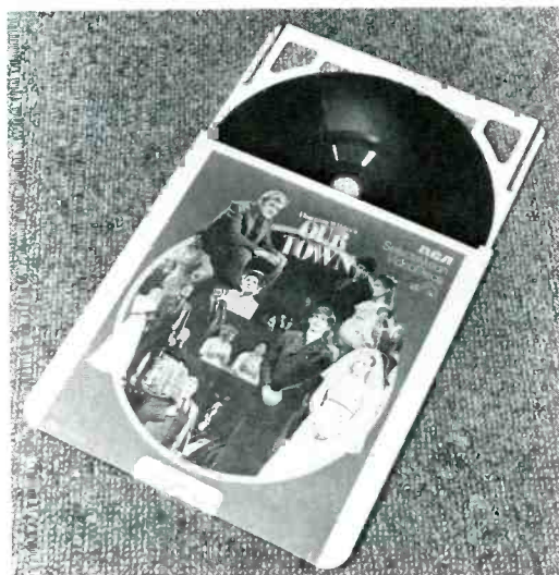
Figure 3. Videodisc caddy. Because of the very small dimensions of the recorded information, the disk is kept in a protective plastic sleeve, or caddy, at all times except when being played in a player. The plastic frame surrounding the disk, called a spine, serves to move the disk into and out of the protective sleeve when the disk is inserted into and retrieved from a player.
