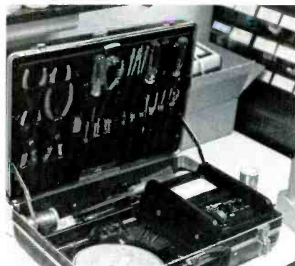
Figure 1 A wide assortment of tools is required for servicing audio-visual equipment. Left, this tool case with its tools is taken on regularly scheduled calls to schools all over the county. Below, another set of tools is kept at the repair shop in a central location.
