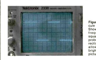
Figure 3 An internal graticule eliminates all parallax. Shown here is the probe frequency-compensation square waveform after the probe was calibrated correctly. The high brightness allows good viewing in bright ambient lighting, as pictured.
