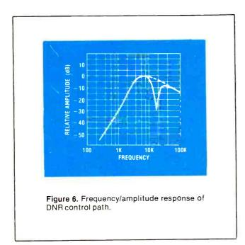
quency, the control path response is increased at 12dB/octave. A careful combination of the low frequency -3dB corner for the high pass filter and the ability to adjust the control path midband gain allows DNR to accommodate a wide variety of music sources.
