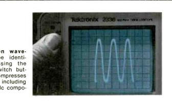
Off-the-screen waveforms can be identified by pressing the beamfinder switch button, which compresses the waveform, including both ac and dc components.
