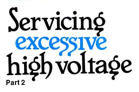
Operation and servicing of high-voltage regulators in solid-state color TV receivers are explained this month.
