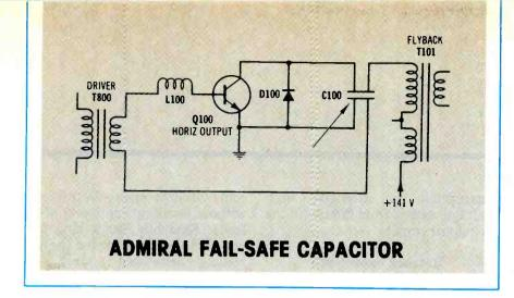
Figure 5 Retrace-tuning capacitors with four leads are used in many color receivers now for safety reasons. If an open occurs in either internal plate of C100, the output stage is weakened or killed, thus preventing operation of the receiver until it is properly repaired. Carefully select a replacement capacitor. See text for details.
