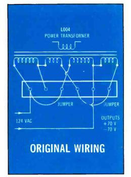
Figure 8 The excessive supply voltages directed suspicion to the power-transformer wiring that had been changed from European voltages. The original wiring, left, had 124V applied to the 110V winding, and one 110V winding fed the other. Right, after rewiring, the 124V of shop line voltage was applied to both *total* 120V windings, with both sections properly powered from the line. The power transformer ran cooler, and the supply voltages were lower after the modification.
