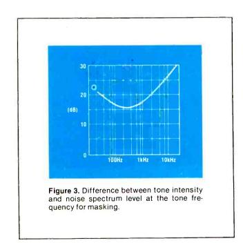
the audible noise and a special spectral weighting filter in the control path ensures that the bandwidth is always increased sufficiently to pass any music that may be present. Because of this ability to analyze the auditory masking qualities of the program material, DNR does not require the source to be encoded in any special way for noise reduction to be obtained.
