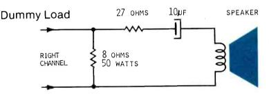
**Figure 4** Because the right-channel amplifier emitted 50V pulses of dc voltage when the erratic noise and amplification occurred, this dummy load was connected to the output. The series resistor and capacitor reduces the ac and steady dc current through the speaker to prevent ruining another test speaker.
