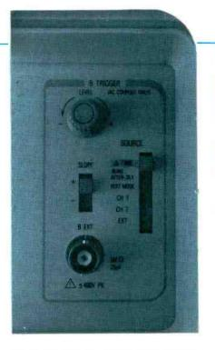
Figure 7 Inside the hinged front cover in model 2336 are the controls for an external B-trigger function (above) and a sliding switch that can select B-triggering or delta-time functions. Located farther to the left (below) is the LCD digital readout that shows the time between intensified zones during the delta-time measurements.
