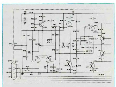
**Figure 2** This is the complete schematic for the right-channel audio amplifier in the 2325 Marantz. In the seven direct-coupled stages, only 10 transistors directly handle the signal and contribute to the voltage and power gains. The other nine are there for thermal and voltage stability. Because of the large number of direct-coupled stages, defects that affect dc voltages are difficult to identify.
