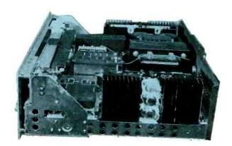
accessible areas cause many problems for technicians trying to perform measurements on individual components. A larger impediment is the common practice of directcoupling several consecutive stages, so the slightest variation of dc voltage in the first stage can saturate the last stage or drive it to cut-off. Defects of this nature are very difficult to analyze and repair. Intermittent symptoms multiply the difficulties.
