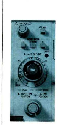
**Figure 5** Controls for sweep mode and sweep times are clearly labeled and placed for easy operation.
