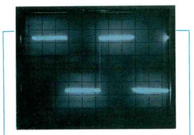
Figure 8 These photographs show the probe-adjustment waveform without and with delta-time trace intensification. Above, in normal sweep mode, the horizontal sections of these square waves are very bright, while the fast rise and fall lines are dim. Below, delta-time trace intensification has brightened the square waves immediately following successive falling edges. Best accuracy was achieved here by moving each intensified area to the left until the falling edge *barely* was brightened.
