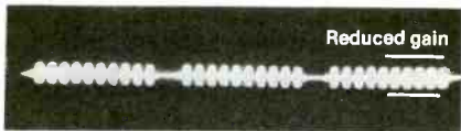
Figure 3b. Symptom: No color. Waveform: Reduced gain at output of bandpass amplifiers.
