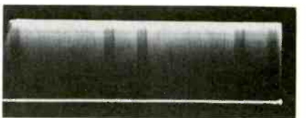
Figure 7d. Symptom: Rolling. Waveform: Vertical sync output of sync separator with vertical sync pulses not present.
