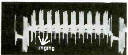
Figure 1d. Symptom: Ringing or ghosting. Waveform: Video detector waveform showing ringing in IF stages or detector.
