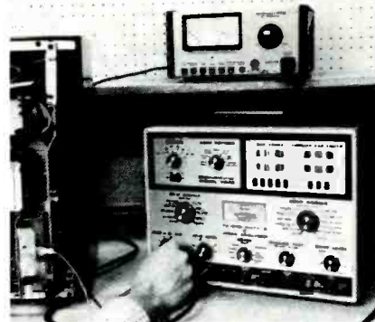
Figure 6. The PR57 isolates the chassis from the ac line while the VA48 is used to substitute for the scan-derived low voltage.
