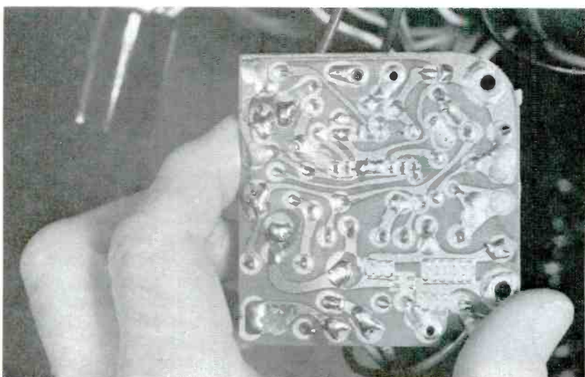
Figure 6 The sequencer circuit board can be unfastened from the frame during measurements. (A) Three screws hold the board in place. At lower-right of the board are seen the three terminals for manual switch and radio receiver. (B) This is a closeup view of the board's top after removal. (C) Wiring side of the board shows etched wiring similar to that in most TV receivers.
