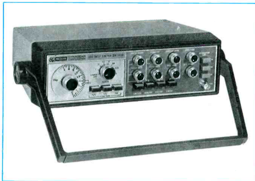
Figure 1 B&K-Precision model 3020 is a 2MHz sweep/function generator with many excellent features, including several functions usually accomplished by pulse generators, sweep generators, function generators and tone-burst generators.
