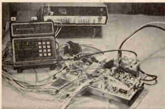
Figure 5 The front-panel selector assembly and the control/tuner chassis of the Magnavox T995 color chassis are shown removed for examination or testing. A microprocessor is incremented or decremented to vary the varactor tuners' tuning voltage until the desired channel is received. This digital code is then memorized for recall when the corresponding buttons are pushed. No variable controls (only push-buttons) are used by the viewer. However, the door above allows technicians access to the programming switches and rotary controls when reprogramming is needed.
