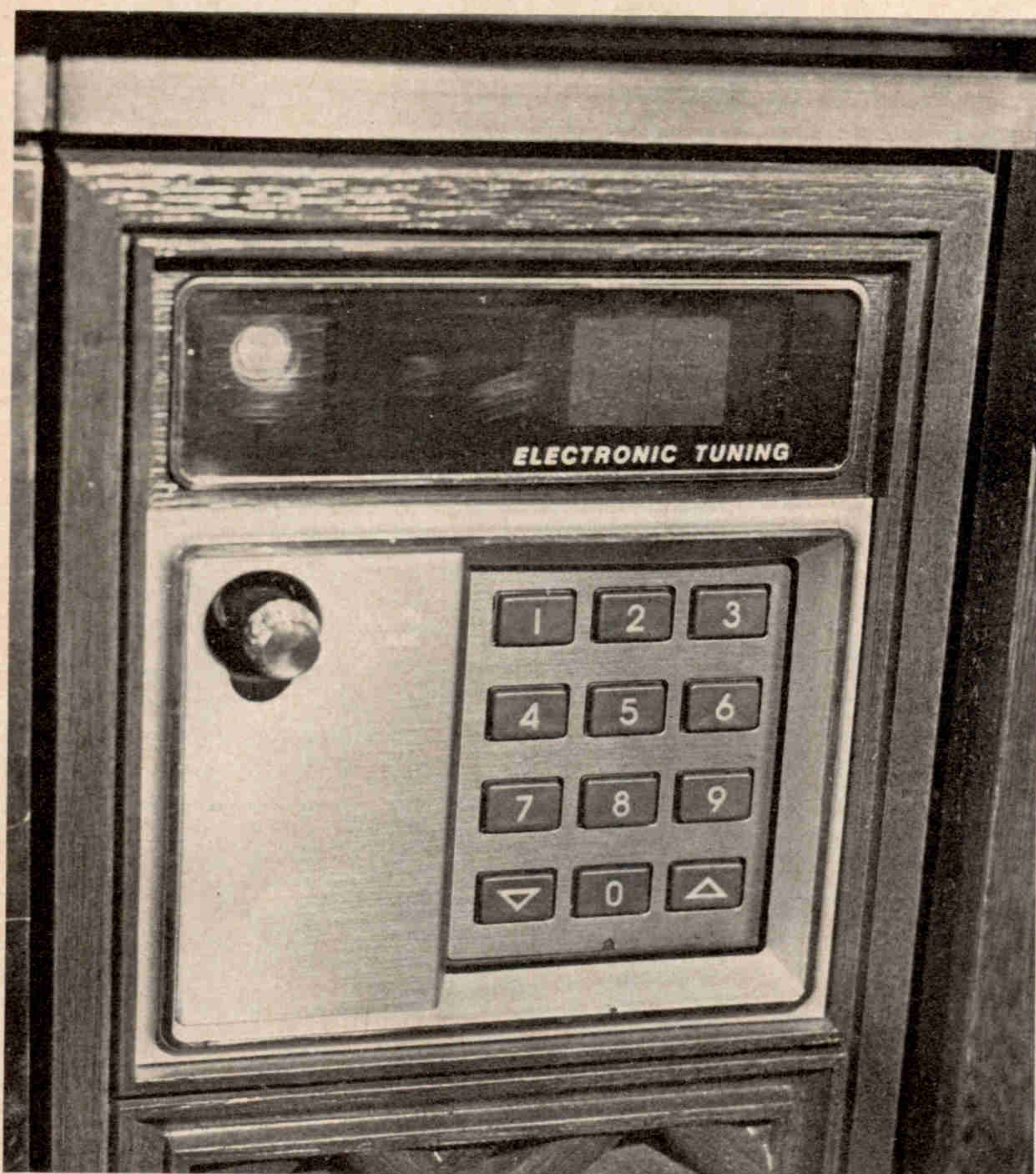
Figure 9 One of the first Quasar color receivers to have frequency-synthesis PLL-varactor tuning operated from this random access push-button keyboard.
