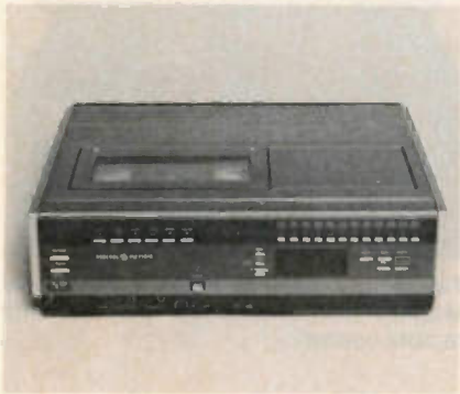
Figure 3 Model 1CVP-2020X is General Electric's first portable videocassette recorder.
