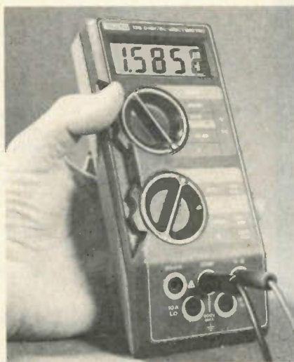
Figure 1 Keithley model 135 features high accuracy with a 4½-digit LCD display using large 0.6-inch digits. Basic Vdc accuracy is \pm 0.05\% + 1 digit. Range and function knobs can be rotated by the left thumb when the meter is held by the left hand, or the knobs can be rotated by the center bar with either hand.
