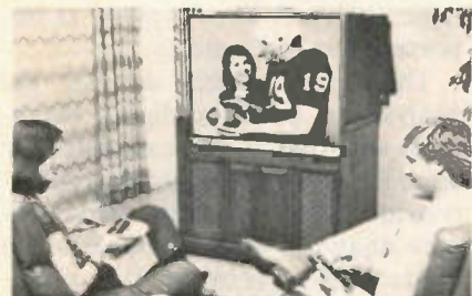
Figure 24 Zenith's model SN-4545P is a projection TV with a 45-inch screen that is hidden when not in use.
