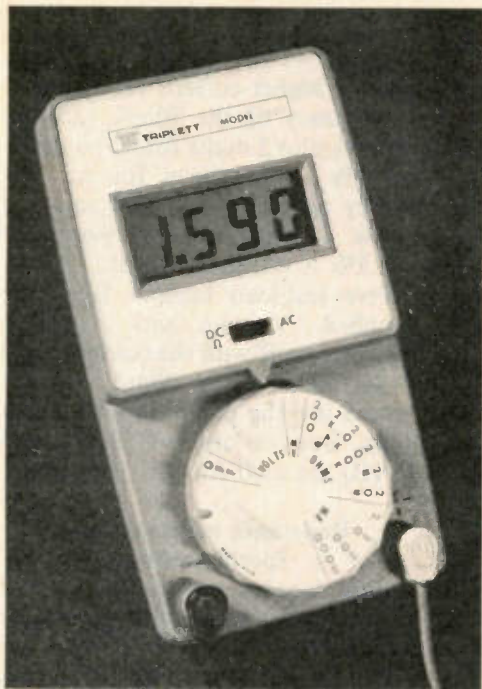
Figure 1 Triplet model 3450 digital multimeter features the essential five functions with more than adequate ranges, plus features such as an audio-response resistance indication and a color-coded selector knob. Simplified controls allow rapid operation with few measurement mistakes. The function-and-range switch has a large knob that turns off the power when fully rotated clockwise. A time-saving convenience is the deletion of all but two test-probe jacks.
