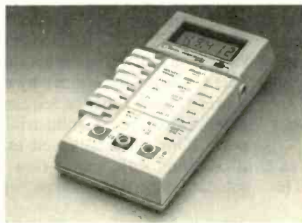
Figure 5 Model 945 from Data Precision does not have an audible tone, but has a basic Vdc accuracy of 0.05% and shows a positive or a negative polarity symbol for decreased ambiguity. Perhaps the most unusual feature is that five of the six ohmmeter ranges can be used to test diodes at decaded currents. Open probe voltage is 3.5V. A specified constant current is applied for each range from 0.1 \mu A on the 20M \Omega range to 1mA on the 2K \Omega range, while the readout shows actual voltage drop across the diode. A list of these five voltages can be made into a 5-point current-versus-voltage curve.
