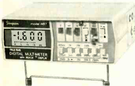
Figure 1 Simpson model 467 has several unique features, including visual and audible indications of continuity, arrows to show a change of signal polarity, true RMS ac readings, pulse identification, and an LCD bar graph to show nulls, peaks and trends.
