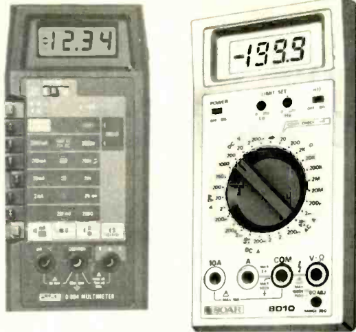
Figure 3 Soar model 8010 has a continuity buzzer, a separate diode test, a shielded case, and basic Vdc accuracy of 0.1%. The distinctive function, however, is testing for high and low limits of reading. Two controls, one for high and one for low, can be adjusted for the allowable limits. If the reading exceeds that range, the buzzer sounds. This is in addition to the usual LCD readout.
