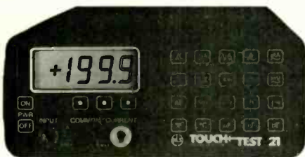
Figure 4 Non-Linear Systems model Touch-Test-21 has 20 functions and 44 ranges selected by internal autoranging and finger touches to the function symbols on the panel. LEDs indicate the function in use. Additional test functions include: an audible continuity indication; a diode test; temperature readings (with probe); conductance readings; and capacitance values.
