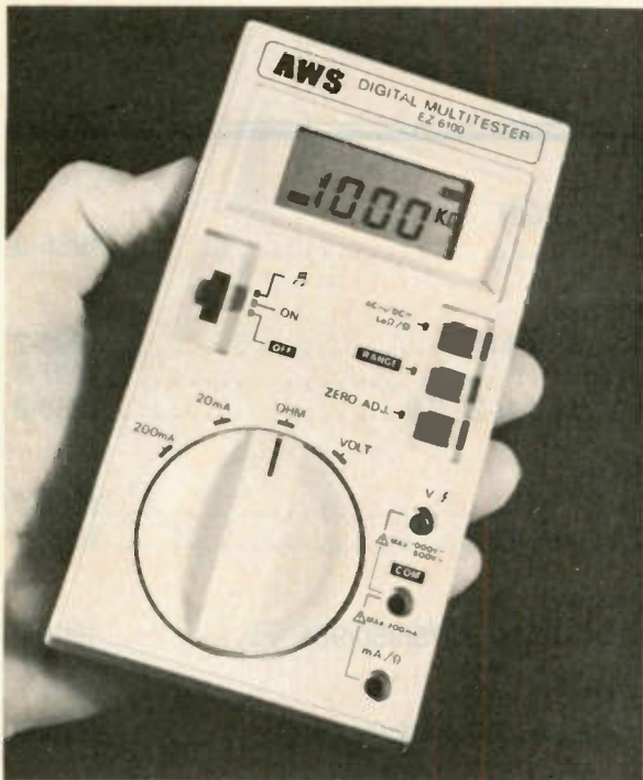
Figure 1 Sperry model EZ-6100 is a small digital multimeter having several unusual features, including additional symbols in the readout, autoranging, and two AA batteries.
