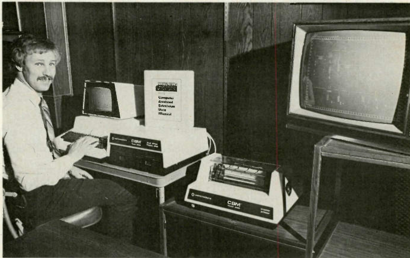
The complete Computech system includes a 32K computer terminal with full keyboard and a small CRT readout, a dual-drive floppy disc, a hard-copy printer and a notebook having about 6500 items of TV parts failures indexed by Photofact numbers. A typical circuit is displayed on the TV screen. H. Lyle McCallister, Computech president, is shown.
