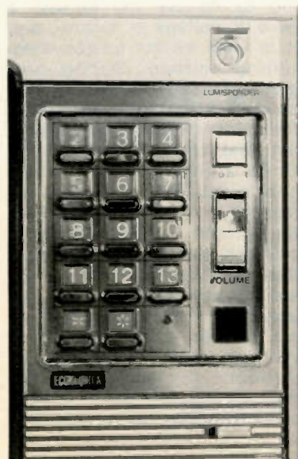
Figure 4 TV channels can be selected either by direct address from the 14 programmable push-buttons on the panel (without up-and-down scanning) or by direct address or up/down scanning of the remote-control unit. After channel selection by either receiver or remote, the appropriate channel number remains illuminated. However, the push-buttons do not latch. The LUMISPONDER CdS cell that controls brightness and contrast is in the upper right corner. Below it is the POWER push-button, which does not latch. A rocker-type up/down audio VOLUME switch provides a slow, gradual change of volume. It is a spring-return type that does not latch. Below the volume switch is the infrared sensor that receives the remote signal. A latch permits the door to open, revealing the programming controls.
