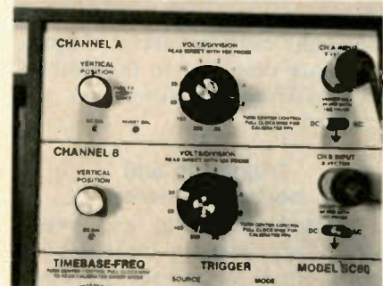
Figure 3 Operating controls for both identical vertical channels are in the upper left corner of the front panel. For calibrated VOLTS/DIVISION accuracy, the concentric variable waveform-height control must be fully CW. Channel A has a polarity-inversion switch operated by the vertical-positioning control.
