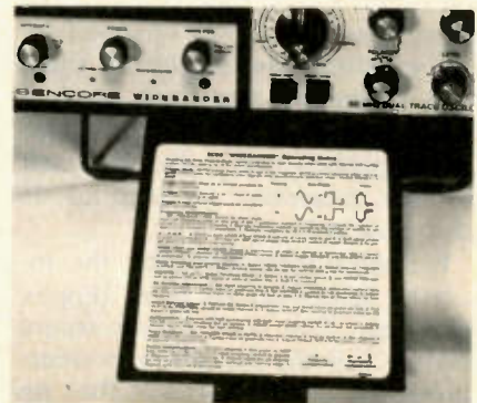
Figure 2 Condensed operating instructions are printed on a pull-out plastic card attached under the scope.
