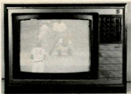
Figure 1 Sony model KV-1543R with chassis SCC-207B-A has 42 transistors, three FETs, 11 integrated circuits and 60 diodes. The RM-503 remote control operates by radiated infrared carrier up to 23 feet.
