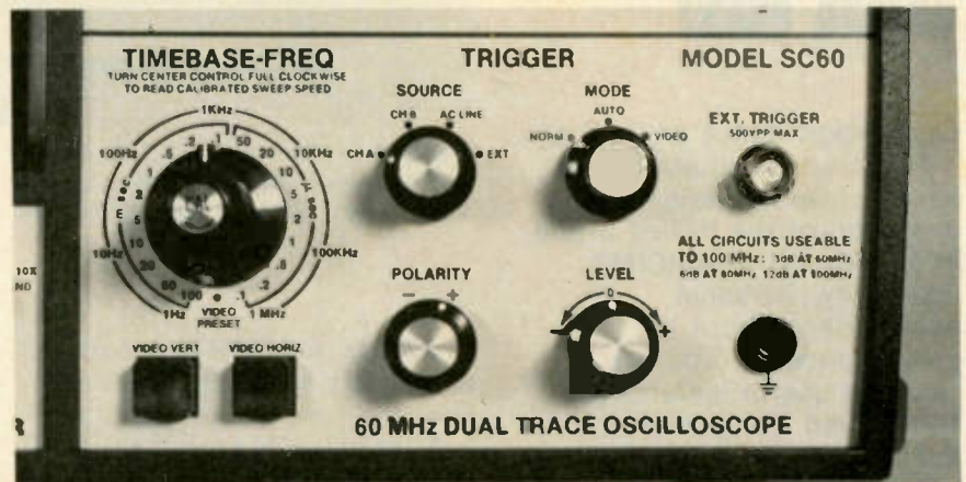
Figure 5 Switches and controls for triggering and horizontal sweep are located on the lower right section of the front panel, along with the external-trigger jack and a ground jack.
