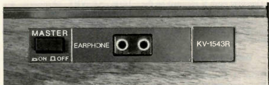
Figure 3 The MASTER power switch turns on and off the dc voltage that powers the remote control. Power to the television power supply is controlled by a relay on the remote circuit board. Turning off the MASTER switch stops all current flow in the TV receiver.
