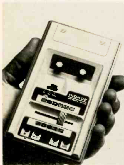
Figure 1 The Hickok model 240 video generator can be held in the hand and the sliding knob of the pattern-selector switch can be moved by the thumb. Both RF and video signals are available from this crystal-controlled video/crosshatch generator.
