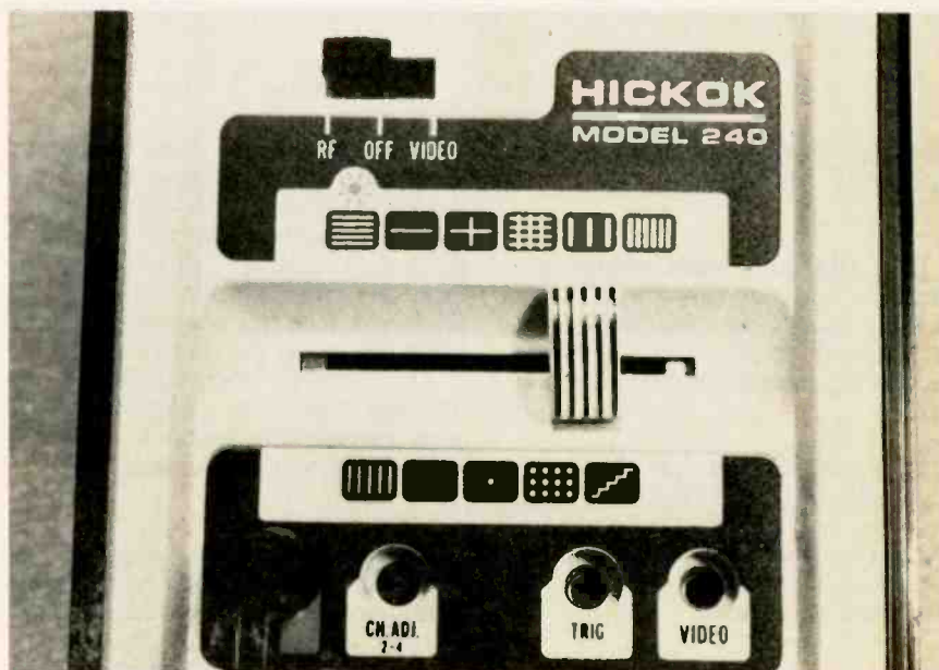
Figure 2 A small reproduction of the pattern marks each detented position of the sliding pattern switch. An LED mounted between the two variable controls lights up on the horizontal-bars position to indicate battery condition. Three jacks and a trimmer are at the bottom. The jacks are for RF, trigger and video outputs; the trimmer adjusts the precise channel carrier frequency.
