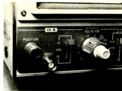
Figure 6 New triggered scopes have some kind of three-position switch that blocks dc and passes ac to the vertical channel (AC), disconnects the probe and grounds the vertical-amplifier input to give zero input (GND) or passes both ac and dc to the vertical amplifier (DC).
