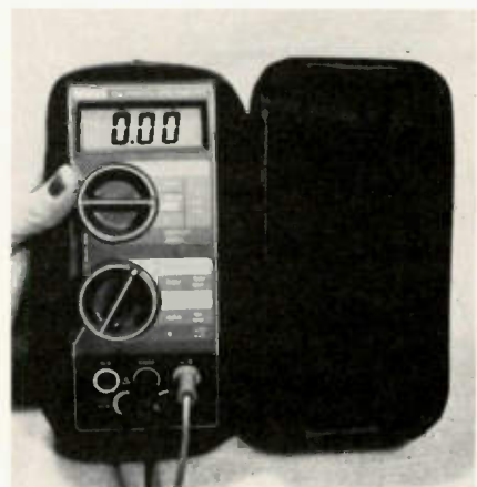
Figure 4 Protection and convenience are afforded by the soft-type zipper-operated carrying case. A large thumb nut holds the meter inside the case (if desired) during operation. A pouch in the lid provides ample space for storage of test probes when the case is zipped shut.
