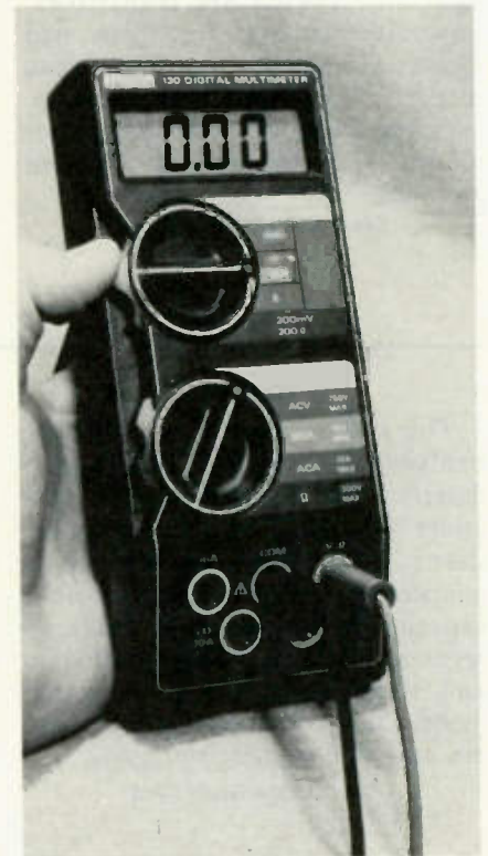
Figure 1 The range switch (top) and the rotary function switch (bottom) of the Keithley model 130 digital multimeter can be rotated by either hand. When the meter is lying down, it is easier to rotate them with the fingers of the right hand on the raised bar in the knob's center. When the meter is held in the left hand, as shown, notches around the knobs permit rotation of the switches with the left-hand thumb.
