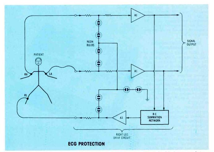
Figure 3 Neon-bulb protection of the ECG preamplifiers and a hum-cancelling drive to the right leg are two features shown by the block diagram.
