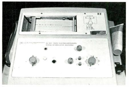
**Figure 5** A typical electrocardiograph is this Hewlett-Packard model 1511. At the right is a tube of conductive paste that is used on the electrodes to give better traces without hum or artifacts.
