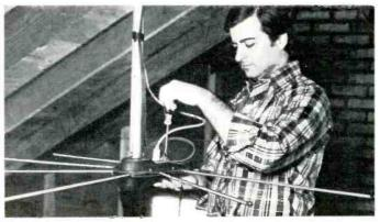
Pictured here is a Winegard 20-20 model. These small antennas are available with or without internal preamplifiers. A combination power supply and rotation control is included. The 20-20 can be mounted indoors or outdoors. The impedance is 75, and a two-wire cable is needed for the power. *Courtesy of Winegard*.
