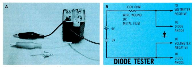
Figure 1 (A) All components are visible in this photograph of the constant-current voltage-drop dlode test adapter. A large wire-wound resistor was used for stability, not because high wattage is required. (B) The schematic is equally simple. Convenience features could be added. An on-off switch and an LED power indicator would remind technicians to shut off the power. A spring-return polarity-reversing switch would save time if many dlode junctions are to be tested quickly.
