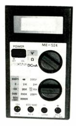
from 200mV to 600V, ac voltages from 200 to 1000V, dc current from 200mA to 10A and resistance from  $2k \Omega$  to  $2 \Omega$ .
