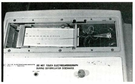
Figure 6 The stylus and galvanometer are exposed for convenient voltage tests and stylus-pressure adjustments after the access cover is removed.
