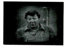
Figure 1 Picture snow can be produced on moderate-to-strong TV signals when the RF AGC negative voltage is too high.
