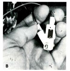
Figure 6 (A) A back-side view of the circuit board that contains the CRT socket shows three power transistors and a few components. Matrixing transistors, drive controls and bias controls are on the main circuit board. (B) The CRT focus pin is a separate assembly that has a large spark gap.
