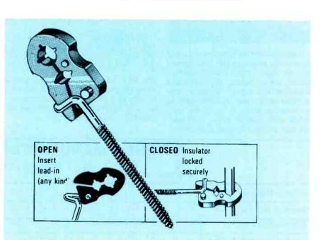
GC Electronics lists many items of hardware for TV-antenna installations. One unique product is E-Z Swing-In standoffs which swing open for insertion of the downlead and then can be locked in the closed position. *Courtesy of GC Electronics*.
