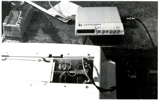
Figure 8 Galvanometer voltage can be measured without removing anything except the access cover. Use an accurate meter, such as a digital multimeter.
