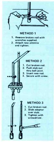
Three methods of repairing the antennas of portable TVs are illustrated in the GC catalog. *Courtesy of GC*.
