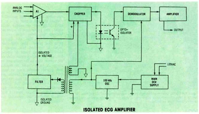
**Figure 4** An opto-isolator transmits ac signals while providing very high isolation between its inputs and outputs. A 100kHz oscillator has isolated windings that furnish ac power for a separate isolated power supply, the isolation chopper, and the demodulator that recreates the original waveform from the pulses sent across the opto-isolator. Therefore, the input preamplifiers and the patient-connecting leads are isolated completely from everything. This is necessary for patient safety.
