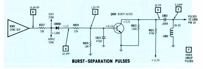
Figure 4 Horizontal-sweep pulses are not used for burst keying. Instead, horizontal sync pulses are processed and used to ring the C803/L802 series-tuned circuit. The important waveforms are shown in the pictures. Waveform D is the driving signal for the C803/L802 ringing circuit. The positive peak of waveform E ringing signal at U800 pin 24 keys-on the burst separation. Figures E and F are dual-trace waveforms that show the ringing-pulse delay (E) relative to horizontal-sweep pulses (F).
