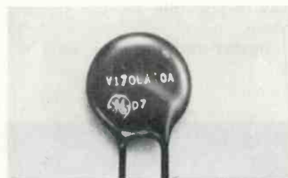
Figure 8 This picture shows the type of metal-oxide varistor used most often for 120V operation in TV sets and industrial controls. When tested for resistance by VOMs and most digital multimeters, a good varistor should read above the highest range. However, a VTVM will show a capacitive kick and perhaps a 100\text{M}\Omega reading. But the best test is to measure the clamping voltage using ac voltage and a scope, as described before. Remember that a varistor minimizes transients by operating as an open circuit to amplitudes below the clamping voltage, or as a very low resistance to amplitudes above the clamping voltage.
