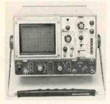
operation, differential measurement capability, and algebraic addition and subtraction of two vertical input signals. The unit operates on 115 or 230 Vac.
