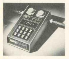
CW or FM power, both forward or reflected, is displayed in watts or dBm. VSWR is calculated continuously and indicated, as is dB return loss.
