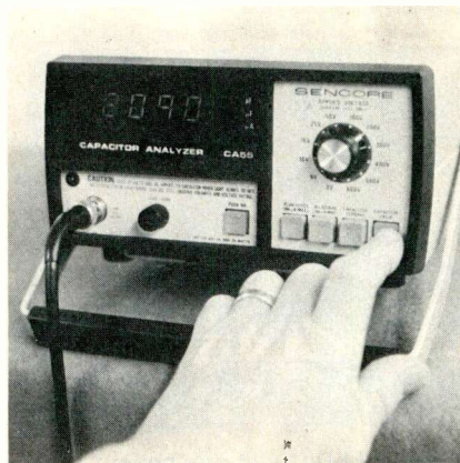
Model CA-55 has the same capacitor tests as the LC-53, but it does not check inductors.
