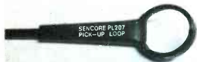
Figure 4 The PL207 RF pickup is small so it can be slipped over coils. The offset handle permits easy location of the loop, even in crowded chassis. This is an excellent method of obtaining a sample signal for the counter, without loading the circuit that's under test, or exposing the counter to excessive voltages.
