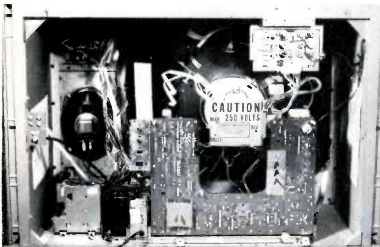
Figure 2 When the chassis is in the normal upright position, the bottom of the "mother" chassis is accessible (picture A). The back of the chassis board (B) has road-map wiring paths shown, plus the markings of many helpful testpoints.
