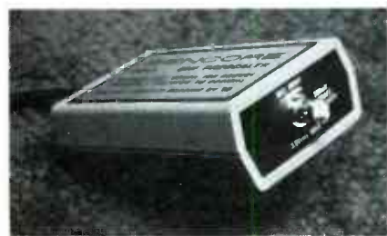
Figure 5 The small PR47 Sencore prescaler permits a counter having an upper limit of 60 MHz to count up to 600 MHz. It has a divide-by-10 circuit. The input is 50 ohms, and the signal should have a level between 300 millivolts and 3.5 volts.
