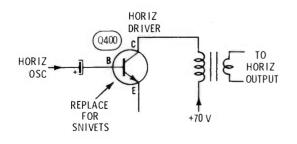
Symptom-Snivets on low channels Cure-Replace transistor Q400, and check snivets
