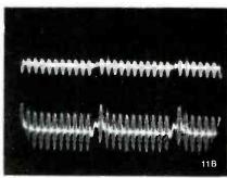
Figure 11 The top trace of (A) is the 0.8-VPP chroma input of M105 at #11, and below it is the 1.2-VPP output at #13, when the Videomatic is off. Turning on the Videomatic activates the LDR, and the output chroma level (bottom trace of B) goes up about 2-VPP amplitude, for normal room brightness.
