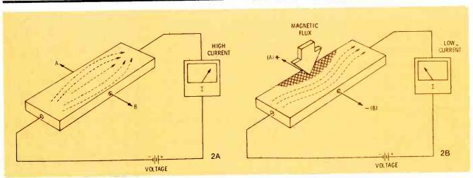
Figure 2 (A) Without flux, electrodes at A and B receive no voltage when the semiconductor passes current. As in Figure 1, the current paths are distributed evenly. (B) When a magnetic flux is applied to one edge of the slab, a
