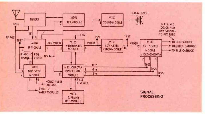
Figure 1 Paths of the IF, video, and chroma signals in the Magnavox T995 color receiver are shown in this block diagram.
