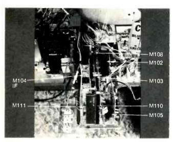
Figure 4 Locations of the signal-processing modules are indicated by arrows. These modules are all on the left half of the chassis.
