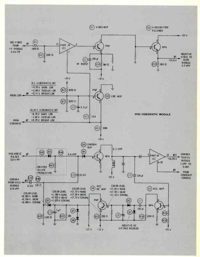
Figure 9 This is the complete schematic of the M105 Videomatic module, which varies the contrast according to the brightness of the room lighting, changes the chroma level in step with variations of the contrast control, and
