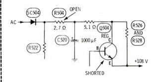
Symptom-No sound, no picture, no raster Cure-Check for open R504 and shorted Q504 regulator transistor
