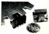
At the left, a Hall-effect transducer senses rotation of the vanes. The sensor at the right shows the two halves, with a powerful magnet on one side and an IC on the other. The vanes block most of the magnetism when they are between the halves. Hall-effect sensors can detect very slow counts (where magnetic devices are useless); that is their main advantage. This unit is rated from zero to 100,000 counts per second. (Courtesy of the Micro Switch Division of Honeywell.)
