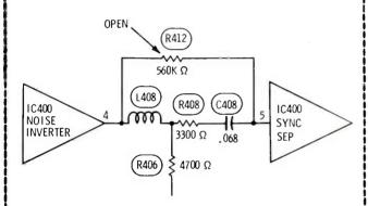
Symptom-Vertical does not lock Cure-Check R412, and replace it if open or increased
