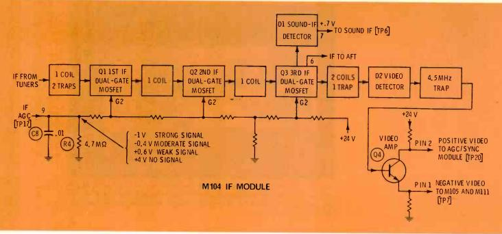
Figure 3 A block diagram of the M104 IF module shows a numbers are given, plus typical AGC voltages produced by conventional array of circuits. Input and output pin various signal levels.
