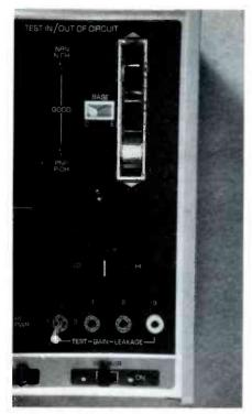
Figure 2 Controls for the in-circuit/ out-of-circuit good/bad and leadidentification tests are located at the extreme right.
