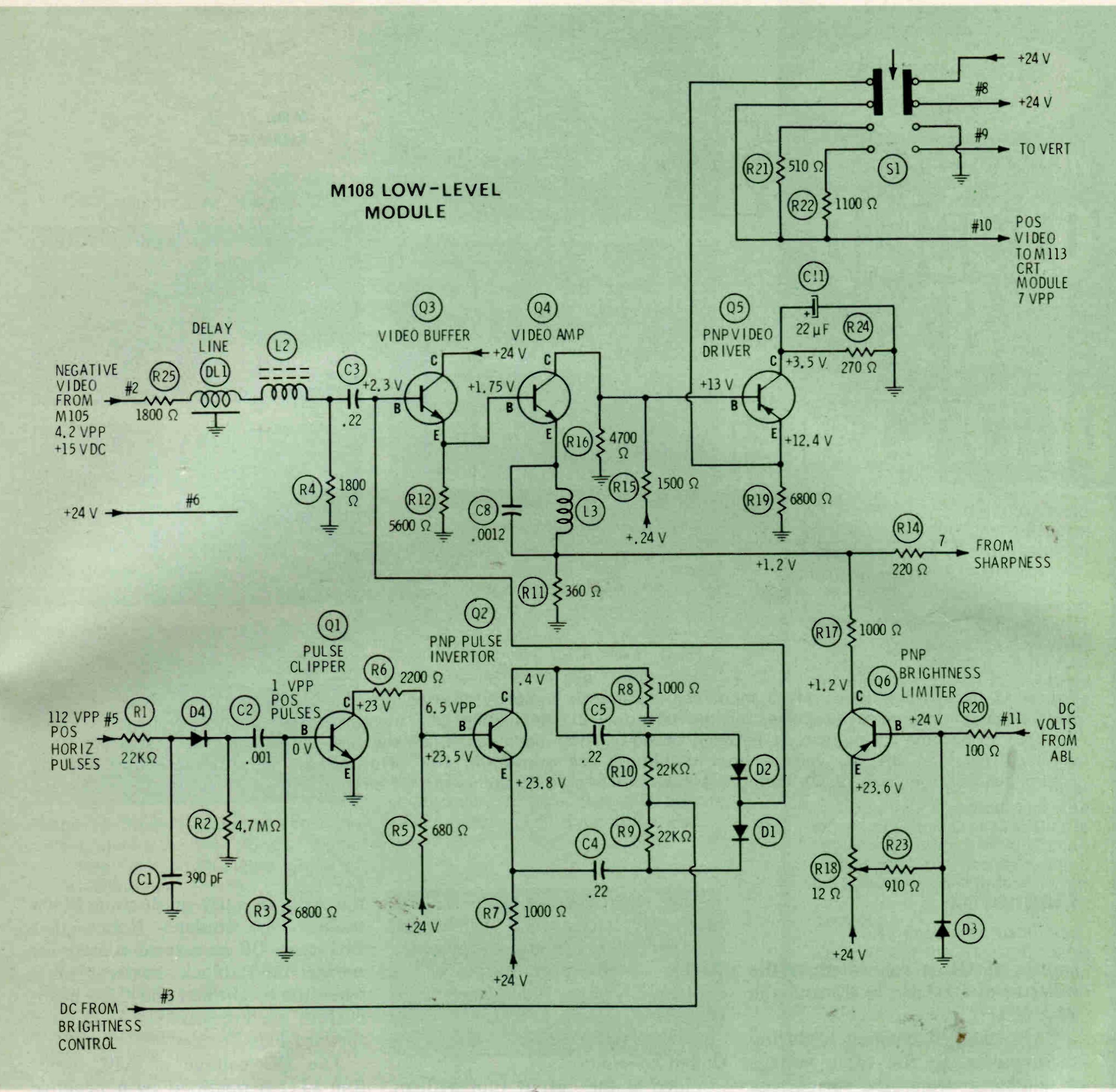
Figure 12 Early-production Magnavox M108 low-level video modules had this schematic. (Figure 13 gives the changes in brightness-limiter and black-level circuits.) Q1 amplifies clipped and narrowed horizontal pulses that have been delayed in phase so they arrive during the back-porch time.
