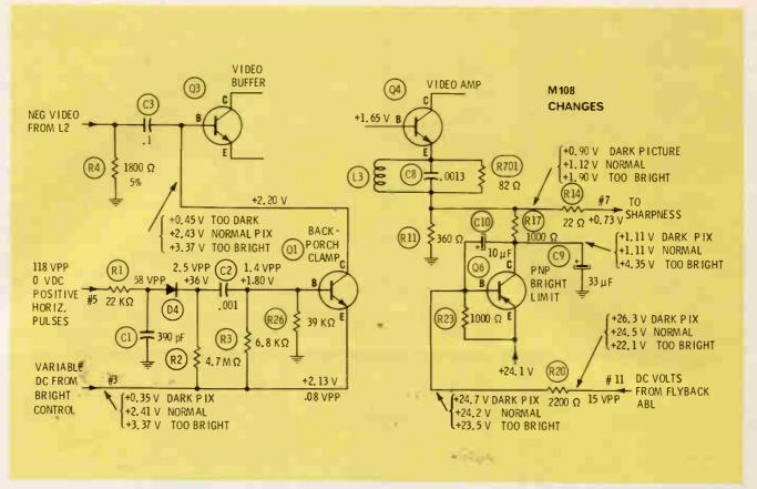
Figure 13 In new-production M108 modules, the narrow positive-going phase-delayed pulses at the base of Q1 force Q1 to become a short circuit between collector and emitter. Therefore, the DC voltage from the brightness control reaches the base of Q3 during the back-porch of
