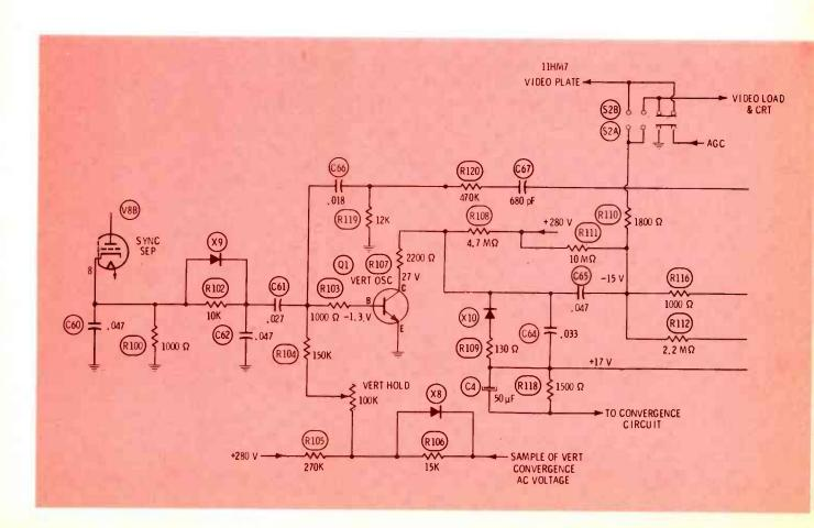
By carefully adjusting the height and linearity controls, I could obtain fair linearity. However, this could not be considered as a satisfactory solution, because the slightest movement of either control brought back poor linearity, and the locking also was too soft.
