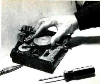
Figure 10 (Top) Remove the flywheel and capstan shaft assembly before you clean out the old grease and apply fresh lubrication to the bearing shaft.
