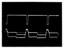
Figure 8 These are the sync-separator waveforms of the M103 module (when the signal was supplied by a model ATC-10 American Technology pattern generator). Bottom trace shows the 9-VPP base input at Q3, while the 25-VPP negative-going sync pulses from the collector are shown at the top.
