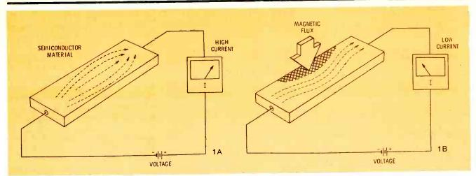
Figure 1 DC voltage applied to a slab of semiconductor material (A) causes paths of the charge carriers (electrons) to be distributed evenly throughout. (B) When a magnetic
