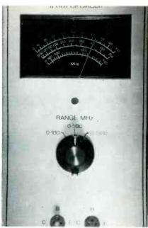
Figure 4 Controls, meter, and circuitry for measuring the frequency where a bipolar transistor gives a gain of one are at the left. They are completely separate from the controls for the other tests. A test frequency of 1 MHz is used for the 100-MHz range; 10 MHz for the 500-MHz range; and 30 MHz for the 1500-MHz range.
