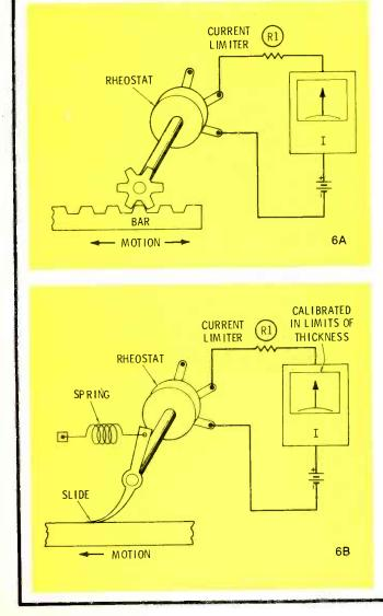
Figure 6 Rheostats and potentiometers can be attached to metal linkages so the lateral position (A) or the thickness (B) of a moving object can be read from the meter.
