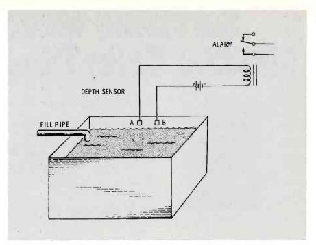
**Figure 8** Some sensors depend on a change of material for a signal. In this example, the liquid readily passes electrical power, and the circuit can be arranged to show overfilling or an empty tank. When the electrodes are in air, the relay has no power. Then, when they are immersed in the conductive liquid, the relay coil is energized.
