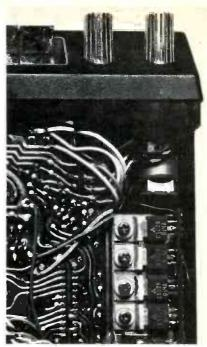
Figure 9 Transistors of this type often develop intermittent operation that originates with the leads. Therefore, move the transistor leads around, using a plastic or insulated tool, and be alert for intermittents.
