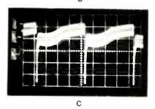
Figure 3 These are the distorted waveforms found before the repair. (A) The sawtooth at the grid of the output tube is flattened. (B) The plate waveform of the output tube also shows the wrong tilt that indicates foldover. (C) Even the waveform at the diode inside the 12JQ6 output tube is badly distorted.
