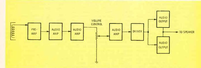
Figure 7 Although signal injection and signal tracing can be done in any stage, most stereo amplifiers divided naturally at the volume control. Inject an audio tone at the volume control and trace each stage to the speaker. Or, inject a small-level tone at the input of the preamplifier and
