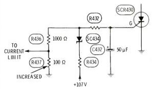
Symptom - Repeated operation of "shut-off" Cure-Check R437, and replace it if increased in value
