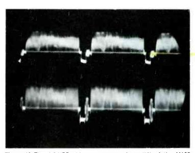
Figure 10 The 4.2-VPP video output waveform (#6) of the M105 Videomatic module (bottom trace) is similar to the 2.4-VPP input (#4, shown by the top trace), except for the high-frequency boost that quadruples the burst amplitude.
