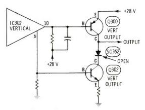
Symptom-No vertical sweep Cure-Check diode SC352, and replace it if open
