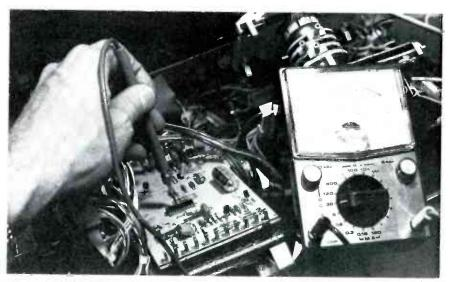
Fig. 7 When high, the outputs of IC201 should measure between +11 and +12 volts. This is an important test of the operation.
