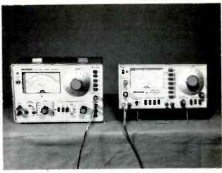
Leader Model LAV-190 Audio Tester and Model LDM-170 Distortion Meter, along with a VTVM or DMM and a scope, are recommended for any kind of audio work.
