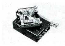
The Model AC-8260, an 82-channel preamplifier, has separate VHF and UHF amplifying stages with a lightning-protection diode and switch-selectable FM trap. Input and output are 300 ohms. Gain is +16 dB on VHF and +17 dB on UHF. Noise figure is -3 dB on VHF and -8.5 dB on UHF.
