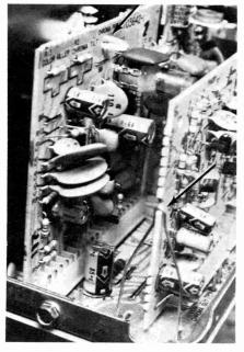
Fig. 8 The modules are held firmly by any two of several methods. As shown in Picture A, the "mother" chassis has sturdy pins which plug into the female sockets on the modules. In addition (Picture B), several modules are snapped over plastic pins (top arrow) which spread to maintain a tension. One or two smaller modules have spring-wire bails that snap into slots in the edges of the board material (arrow at the right center). Some modules are fastened by metal screws.
