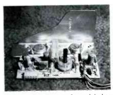
Fig. 11 The power-supply module has two voltage-regulating stages; one is for the +120-volt supply, and the other regulates the +24 volts. Also, Q5 adds a 4.5-volt parabolic waveform to the regulated +120 volts to narrow the picture at the top and bottom (eliminates pincushioning).
