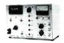
The unit also includes a built-in 12-watt dummy load and an RF power-output meter with a 0-10 watt peak-reading meter for modulation check. The fifth function is a  $3\frac{1}{2}$  digit .05% DVM that can be switched to read power-supply voltage, or used externally to read .01 to 19.99 volts for transceiver probing.
