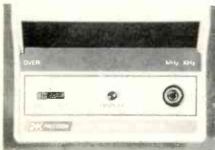
Fig. 3 Only three controls are on the uncluttered control panel. The three LEDs for the "over" "MHz" and "KHz" indications are under the dark anti-glare window, along with the six digits.
