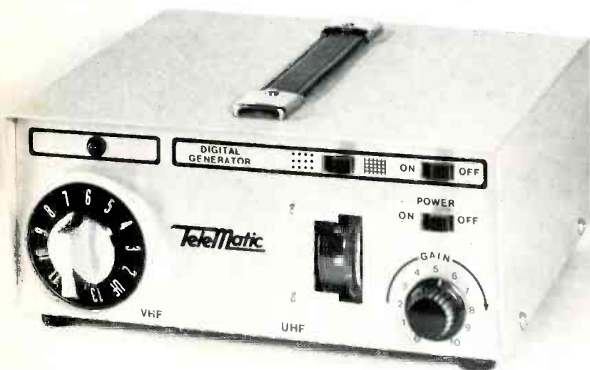
Fig. 1 The TeleMatic "Ferret" not only provides VHF and UHF tuners for substitution tests, but also has a generator of crosshatch and dot patterns.
