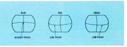
**Fig.** 4 Viewed on the screen, all of the crosshatch lines are curved, except for the blue-vertical lines. They are not bent, because the blue gun is midway between the vertical yoke coils (which are at the right and left sides).
