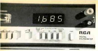
Fig. 2 This photo shows the unretouched 0.45-inch LED display, and the pushbutton operated switches, including those for the separate 20-megohm resistance range, the "LP" ohmmeter voltage, and the low-range millivolt, microampere, and 200-ohm functions. (This instrument has the RCA name.)
