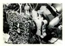
Fig. 18 Picture tubes with in-line guns typically have simplified convergence adjustments and components. This GE convergence assembly has four rotary magnets for center converging the red and blue with the green. Most of the dynamic convergence comes from a special winding inside the deflection yoke. inside deflection-yoke covers, as pictured in Figure 16B, have been known to bind against the plastic, thus they were prevented from touching the glass neck.
