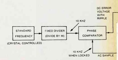
voltage (positive to the cathode). Consequently, a fixed positive bias is added to the variable-polarity voltage from the comparator. Following filtering of the errorcorrecting DC voltage, the voltage at the varicap diode might swing from near zero to about 6 or 7 volts, according to the amount of frequency error, with phase-lock occurring at about +3.5 volts.
