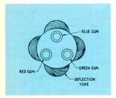
Fig. 3 Each gun of the delta tube is off-center in the yoke. Therefore, the crosshatch lines will be curved.
