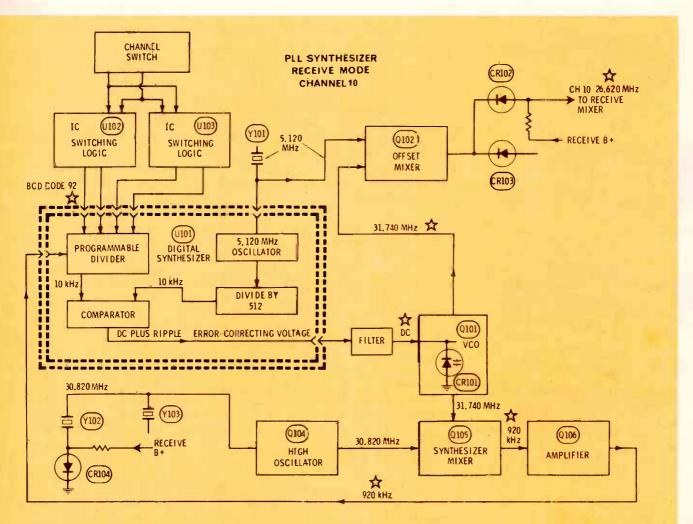
Fig. 7 The receive-function block diagram is the same except for the Channel 10 receive frequencies, and the diode keying of the high-oscillator crystal and the output from the offset mixer.
