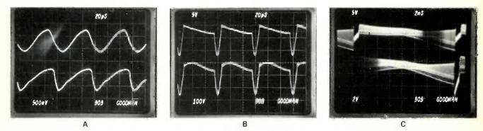
Fig. 15 One test of a convergence control or coil is to attach the scope probes across the terminals and adjust it. The waveforms of (A) were found across T601 when R601 was turned from one end to the other. (B) shows the waveform of L601 at the two extremes of adjustment. The waveforms of (C) were taken at the end adjustment of R618, when the scope was across T601.
