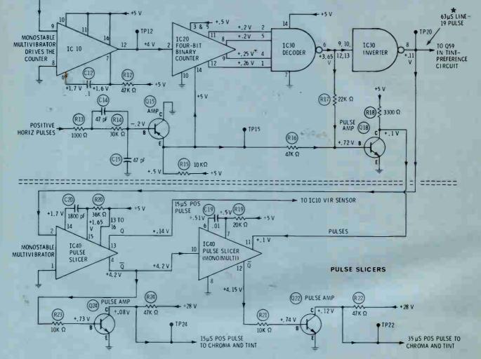
Fig. 9 The use of IC's, whose internal components are not shown on a schematic, makes this full diagram of the Line-19 Identifier and Slicer stages seem less formidable. Therefore, the circuit operation is not difficult to understand.
