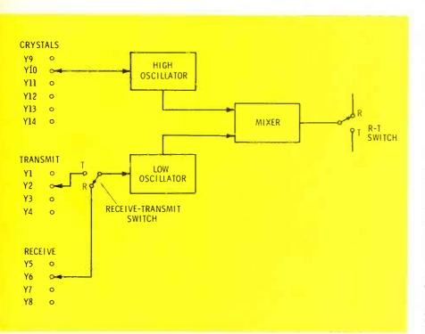
**Fig. 2** Heterodyne frequency synthesizers were developed to reduce the number of crystals (46) that previously were necessary for 23 CB channels. By combining in a mixer stage the RF outputs of two crystal oscillators, extra sum-and-difference frequencies are produced. A proper selection of 14 crystals can supply the 46 frequencies necessary for receive and transmit of 23 channels.
