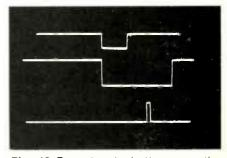
**Fig. 12** From top to bottom are: the 520 microsecond pulse at TP10; the 1400 microsecond pulse at TP12; and the 63 microsecond Line-19 pulse.
