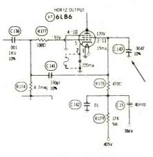
Finally, I checked the DC voltage at the screen grid (should be 120 volts), but found only about 25 volts. I tried three separate output tubes, but with no change of symptoms. However, an ohmmeter test showed only about 1,000 ohms from the screen (pins 3 and 11) to ground. Of course, that's much too low. I removed the output tube from its socket, and short was gone.
