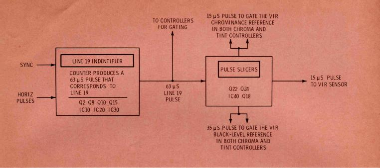
Fig. 8 The block diagram shows the stages we will examine this month. A combination of transistors and IC's, as well as both linear and digital techniques, are used throughout the VIR stages.
