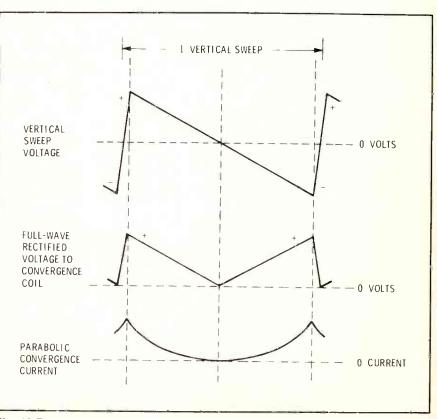
**Fig. 10** These drawings show the operation of the circuit of Figure 9, explaining how one positive and one negative peak combine to make two positive peaks. In turn, those peaks produce a near-parabolic current.
