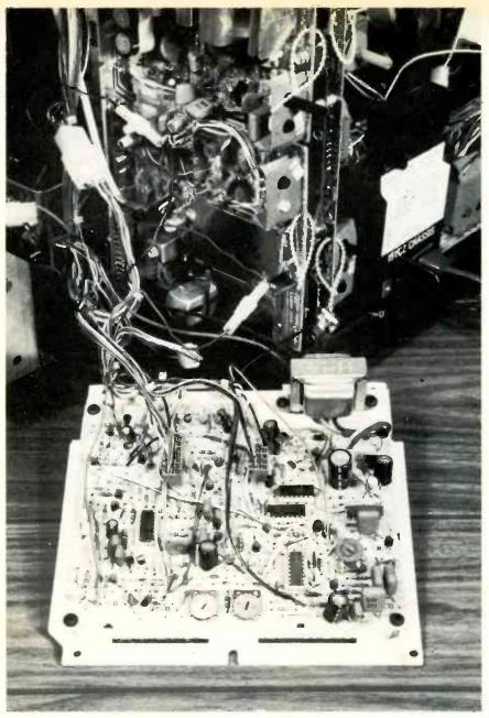
Fig. 7 Wires to the many plugs and connectors are long, allowing the module to be positioned behind the main chassis, when examination or testing is needed.
