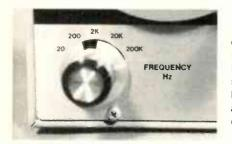
**Fig.** 5 Limits of each range are indicated by a slit in the knob which shows a black bar between the low and high frequencies.
