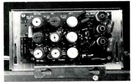
Fig. 6 This is the convergence circuit board of a 25" color tube. The six controls on the left are for vertical convergence. The three controls and three coils on the right are for horizontal adjustments.
