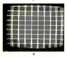
Fig. 17 Picture (A) is a normal crosshatch pattern on a new General Electric receiver that uses an in-lineguns picture tube. When the convergence coil was shorted out, the horizontal lines of the crosshatch (B) were not affected.
