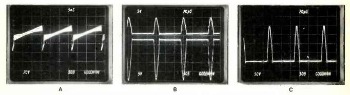
**Fig. 14** These are the four input waveforms to the convergence board of a Zenith 19EC45 chassis. (A) Vertical-sweep sawteeth (with butterfly wings from the pincushioning) of about 55 VPP enter at pin 6. (B) The waveform at top is the 8.8 VPP horizontal pulses at pin 7, while below are shown the 27 VPP negative-going pulses at pin 2. (C) More positive-going pulses of 200 VPP are found at pin 4 of the convergence plug.
