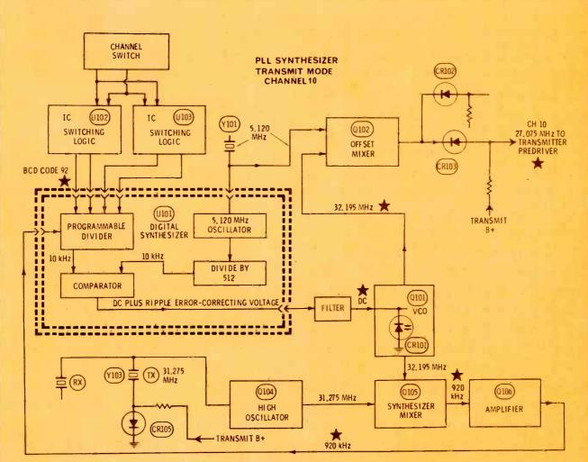
**rig. 6** This E. F. Johnson PLL has the same general circuit as the one in Figure 5. It is drawn differently because several basic stages are inside U101 Integrated circuit. The frequencies are the ones for transmit on Channel 10, and the ones with stars are different for each channel.
