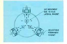
Fig. 1 The center-convergence permanent magnets of delta-gun picture tubes are mounted with the dynamic convergence coils. Rotating or sliding a magnet in its holder varies the magnetic field, which moves the entire picture of that color, Red and green can only intersect at one point near the center; then blue is moved up or down and sideways to converge.
