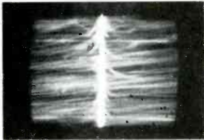
Fig. 7 At low brightness the RCA CTC63 chassis would develop a parasitic oscillation that appeared as a jagged line down the center.
