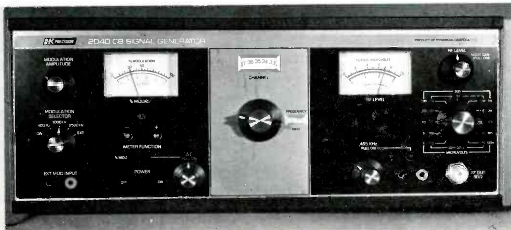
Fig. 1 Controls of the B&K-Precision Model 2040 CB Signal Generator are laid out logically, to speed operation and minimize mistakes. Modulation controls and meter are on the left, channel selector is in the center, and attenuation controls, meter, and RF/IF output jacks are located on the right.
