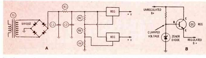
Fig. 3 Regulation of some voltage sources improves both the regulation and the filtering. In schematic (A), the regulator circuits are shown by boxes, while (B) gives a typical series-transistor regulator circuit.
