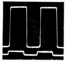
Fig. 5 The top waveform shows the normal 3-VPP drive signal at the base of Q400, horizontal driver transistor; and the lower trace is the small signal there after the SCR has conducted.
