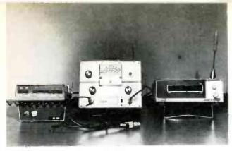
Fig. 3 The 3-inch stub of cable with connector was disconnected from the counter, causing a 1/2 watt loss of power when it was left open.
