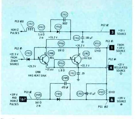
Fig. 5 These three voltage sources are located on the power-supply module. Notice that all three receive their power from the horizontal-sweep circuit, although the regulated source is stabilized from the + 22.5-volt source, which is powered from the main B + source.
