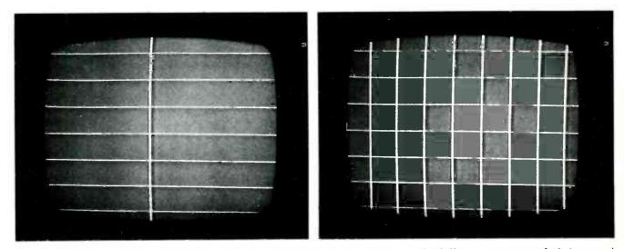
Fig. 2 Separate switches allow a selection of none, 1, 3, or 11 vertical lines or rows of dots; and none, 1, 3, or 7 horizontal lines or rows of dots. Both switches at "off" give a blank raster. These are two of the 18 possible patterns from Model 431.
