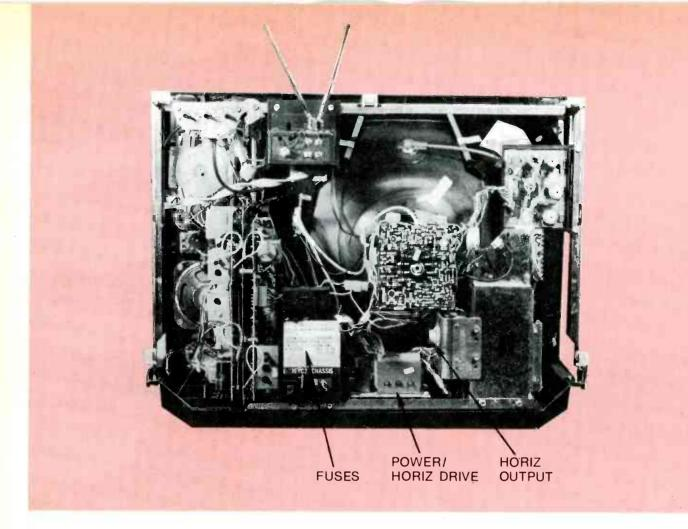
Fig. 1 Locations of some power-supply components are shown here.
