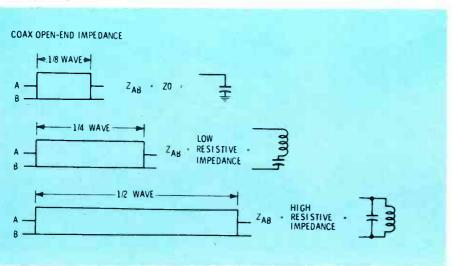
Fig. 1 When it isn't loaded properly, coax cable acts as a short or an open circuit, depending on the length of cable and the frequency. An open-ended piece of coax acts as a capacitance when the length is 1/8 wavelength. At 1/4 wavelength, the input of the cable has a low resistance. When it is 1/2 wavelength, the cable appears to be a high resistance.
