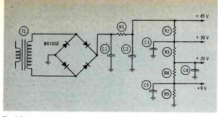
**Fig. 2** Some power supplies furnish voltages for the power amplifier, as well as for the oscillators and gates, by means of a voltage divider.
