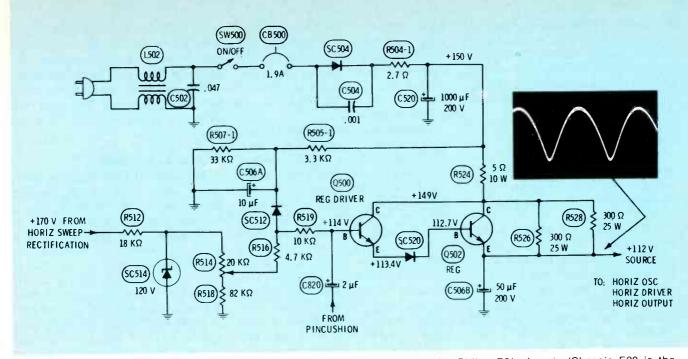
Fig. 1 This is the schematic of the main power supply and regulated source for Philco E21 chassis (Chassis E20 is the same, but the supply is set for  $\pm$  107 volts). The parabolic waveform should be found at the base and emitter of Q500, also the base and emitter of Q502. Operation of the regulator can be understood more easily if you eliminate Q500 and connect the base components to the base of Q502.
