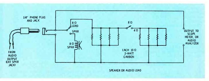
Fig. 6 Build this audio load circuit in a box with the test speaker. Measurements made with the 8-ohm dummy load are more accurate and easier on the ears. The output terminals are convenient points to connect test equipment.
