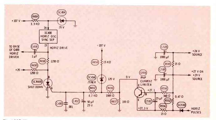
**Fig. 4** SCR430 shorts out most of the signal intended for the horizontal driver when either the +112-volt regulated voltage is too high, or the current of the +29-volt source is excessive. Either defect makes the gate of SCR430 positive, and it conducts until the power is turned off and the voltages are discharged. Loss of the drive eliminates the high voltage and the +29-volt supply, giving no raster and no sound.
