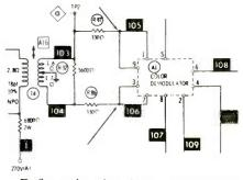
Defects in the ACC and killer circuits sometimes produce some odd symptoms, so I checked there. Sure enough, the killer could not be made to develop -23 volts, and the collector of the ACC transistor was far from the usual +75 volts. Both transistors checked normal.
