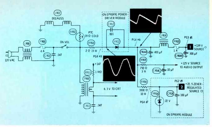
Fig. 2 One diode (Y912) rectifies the power-line voltage; others operate from horizontal-scanning power. A heater transformer for the CRT is supplied, but no power transformer. Those components enclosed in dotted lines are on the powersupply/horiz-buffer module. Others are on the power/fuse bracket, or mounted on the chassis frame. The positive peak of Y912 anode waveform is flattened because of the voltage drop across R904.
