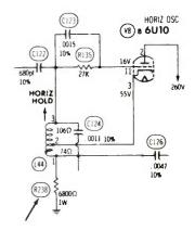
Evidently, the wrong value had stopped the oscillator, because replacing the resistor restored normal operation.
