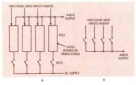
Fig. 1 Audio from the tone generators either is keyed by some kind of gate (A), or directly by the key switches (B). A DC supply is required to operate the gates, which might be diodes, transistors, neon bulbs, or tubes.
