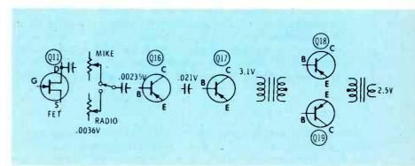
Fig. 7 These 1,000-Hz signals of the amplitude shown should produce an output of 2.5 volts RMS from a Johnson Model 124, during signal-injection tests.
