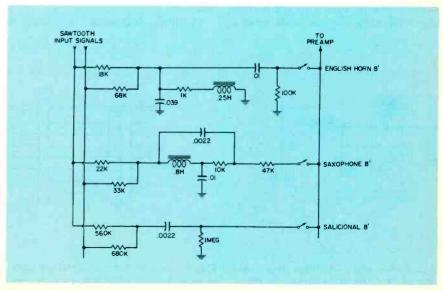
Fig. 4 These are examples of the stop filters used in some models of Baldwin organs.
