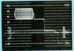
Fig. 1 The new VIR signal waveform is shown here both as a drawing and the way it appears on a scope screen, direct from a VIR generator. TV stations can use it to correct many video and chroma distortions. Some General Electric TV receivers now automatically adjust both tint and color saturation, when the VIR signal is broadcast.
