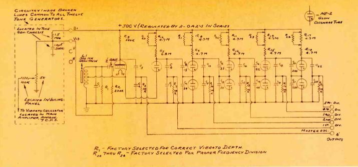
Fig. 12 Kinsman organs are unique for using neon bulbs in the dividers. One generator of six octaves is shown in the diagram.
