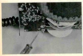
Fig. 8 Only one connection requires unsoldering.
