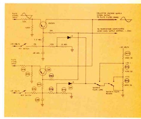
Fig. 8 The flute output from each Conn oscillator is keyed by changing the bias of a transistor, as shown. C26 delays the change of bias voltage to eliminate any clicks, and a fixed voltage through D4 determines the sustain time before the note dies away.
