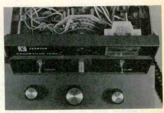
Fig. 7 The knobs slide off the flattened shafts, exposing the nuts on the controls. The large nuts, and two screws at each edge of the panel, must be removed to free the front panel.
