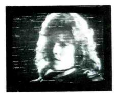
Fig. 8 Noise that isn't synchronous with either the vertical or the power line appears at random, without any pattern. This noise was made by a brush-type motor.
