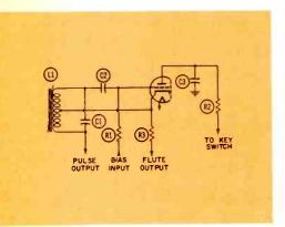
Fig. 5 R2 and C3 filter the plate voltage of Conn oscillators, to eliminate clicks, and to make the attack and decay times more natural.
