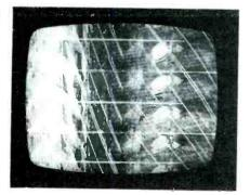
Fig. 2 If the vertical is locked correctly and then the sync is eliminated, does the vertical sweep run faster or slower? Truth is, the sync should force the oscillator to fire ahead of time; therefore, a loss of sync makes the sweep run slow (flips upward rapidly).
