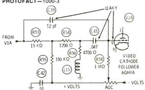
Symptom—Video blanks out, requiring adjustment of AGC
