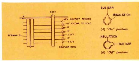
Fig. 6 Many switch contacts are under each Conn keyboard. Depressing a note makes contact when the coupler rod is turned with the metal side toward the key-switch finger. The note cannot play when the coupler rod is turned with the insulation toward the switch wire.
