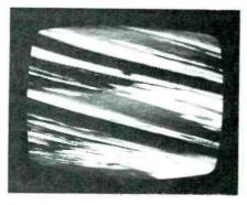
Fig. 14 When the horizontal-sweep frequency is too high, the black bars of the horizontal-blanking bars in the video slant downhill to the right. Remember it as a signal going faster downhill. Each black bar represents a frequency error of 60 Hz; therefore, the frequency here is 15,914 Hz.
