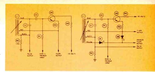
Fig. 7 These two examples of Conn oscillators show how two waveforms are obtained from one type, and three waveforms come from the top-octave type that has diodes acting as a doubler. These oscillators operate continuously. The pulse outputs are keyed directly as audio, while the flute outputs are keyed by transistors, with one transistor per note.
