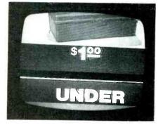
Fig. 1 When the picture and blanking bar move slowly down the TV screen, is the vertical sweep too slow so the video moves ahead of it on the way to the bottom of the screen? Or is the sweep too fast and moves part way to the bottom before the blanking bar arrives?
