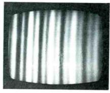
Fig. 12 Defects in the horizontalblanking circuits (usually bad diodes) can allow the ringing between pulses of the high voltage to come through the video amplifiers, causing vertical bars.
