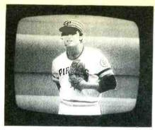
Fig. 6 These shaded areas have been called "silicon-diode radiation", but that's wrong. Instead, they are modulation bars caused by a change of signal strength from conduction of the power-supply diodes. They can't be seen unless there is a carrier which can be modulated.
