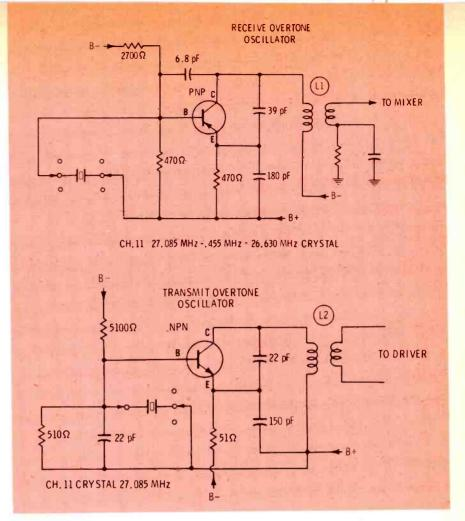
Fig. 2 These are two typical oscillators using a third-overtone circuit.
