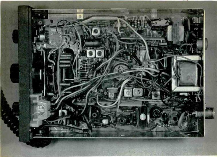
Model 123A CB radio from E. F. Johnson (Photofact CB-47) is used as an example of modern synthesizer design.
