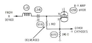
Symptom—Herringbone pattern in red picture Cure—Check R191, and replace if it is reduced in value Chassis—Truetone MIC-4212-27 PHOTOFACT—1265-2
