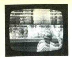
Fig. 3 A vertical roll that happens regularly every 16 seconds is caused by a certain kind of hum.
