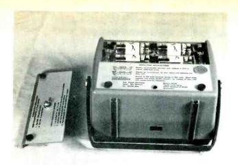
Fig. 6 Larger size of the DVM32 permits operation from four "C" cells, thus allowing longer operation before battery replacement. An adapter is used when line power operation is desired.
