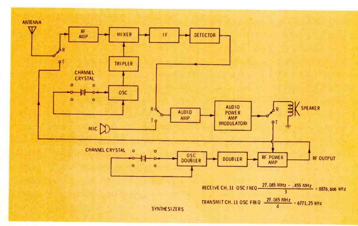
Fig. 1 A block diagram illustrates an older CB transceiver with separate oscillators that operated at low frequencies which were doubled or tripled to reach the CB band.
