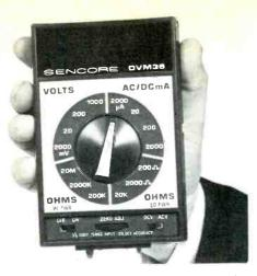
Fig. 4 Although the DVM36 appears to be nearly identical to the DVM35, it has  $3-\frac{1}{2}$  digits, permitting overranging up to 1999 instead of stopping at 999, and has a basic accuracy of 0.5% for DC voltages.
