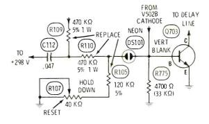
Symptom—Intermittent vertical jitter Cure—Check R105, R109, and R110. Replace if out of tolerance, and readjust R107
