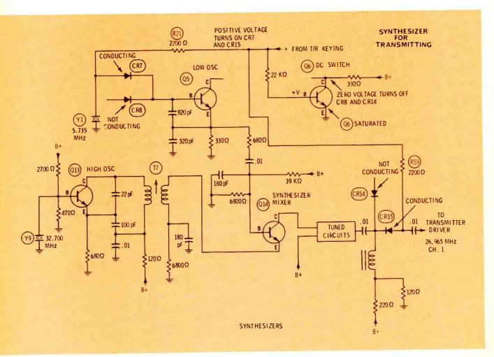
Fig. 5 This schematic shows the same synthesizer with switching and signal flow in the transmit condition. Positive voltage from the mike switch forces CR7 to conduct, connecting the base of Q5 to the low-frequency transmit crystal that has been selected by the channel switch. The same voltage keys-on CR15, which feeds the output of the synthesizer to the transmitter driver stage.
