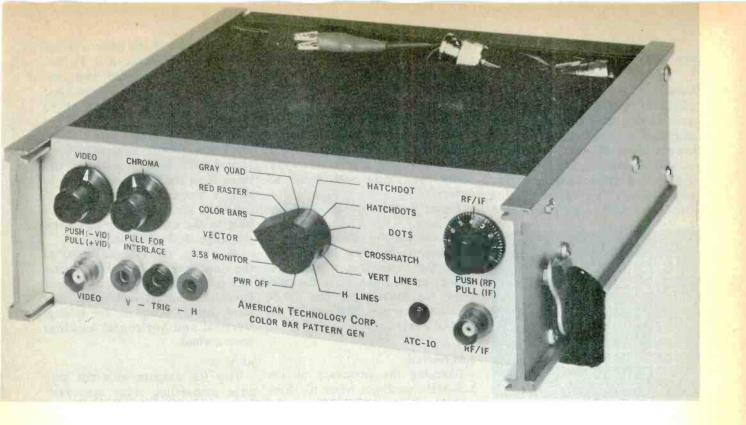
ATC-10 allows you to obtain the red screen in the same way as is done by the TV station. In other words, the generator provides the proper phase of chroma signal, which will appear as pure red when the set is normal.
