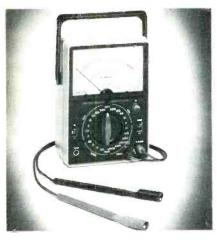
Model 60-NA is drop-proofed for an accidental drop up to five feet. Three fuses provide burnout-proof protection for the meter. It has a suggested price of \$130.
