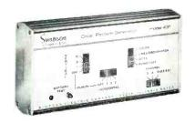
purity adjustment, single dot and single crosshatch for static convergence and centering, 11 vertical lines for horizontal linearity, 7 horizontal lines for vertical linearity, 3X3 dots and 3X3 crosshatch, 7X11 dots and 7X11 crosshatch for dynamic convergence. The 431 tests for gray scale tracking, overscan, pincushion, and AGC.
