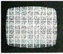
Fig. 11 The carrier-signal attenuator, which is marked "RF/IF," can reduce the signal an unusual amount, because of a special circuit with double shielding. AGC, snow, and other problems can be checked by the ability to select any signal strength that's necessary to trigger the trouble. As shown here, the signal can be attenuated until it is about equal to the snow of a good TV receiver.
